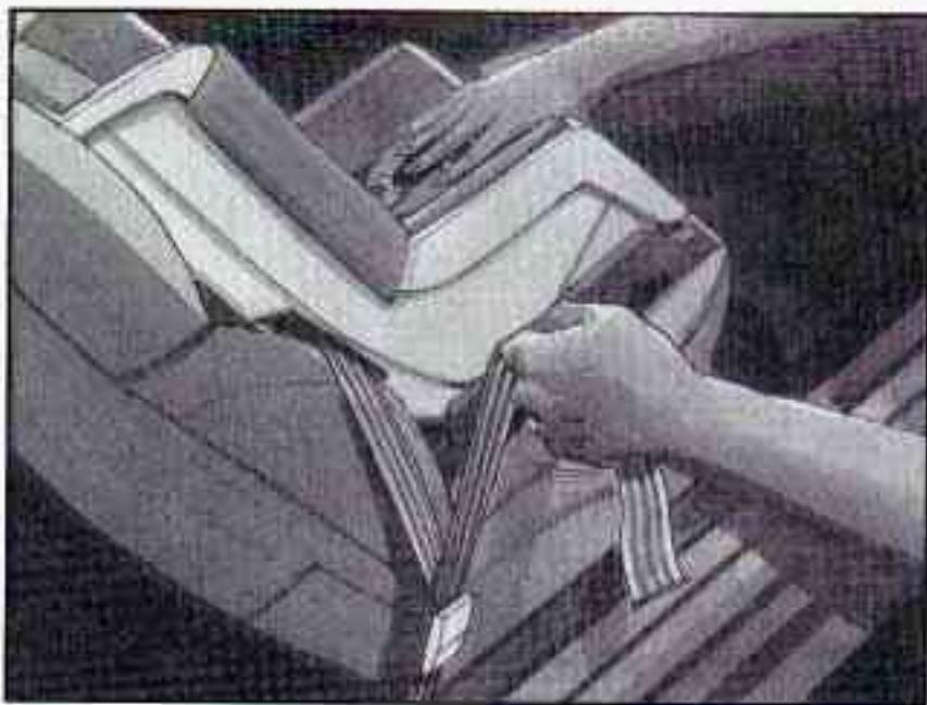
10. Push and pull the child restraint in different directions to be sure it is secure.
