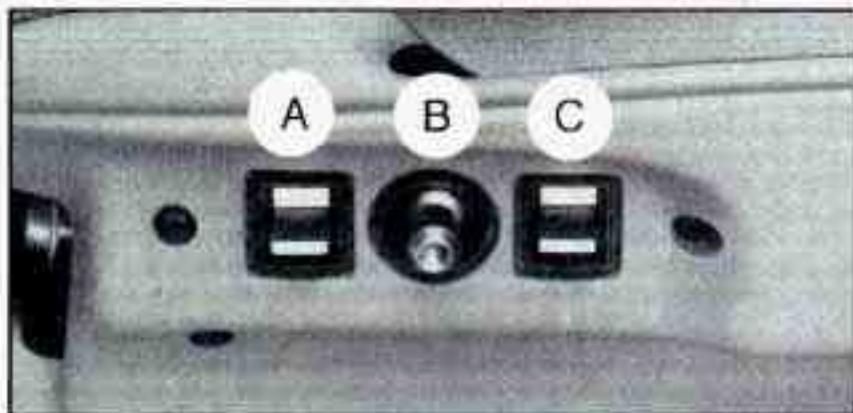
**FRONT (A):** Raise the front of the seat by holding the switch up. Hold the switch down to lower the front of the seat.
