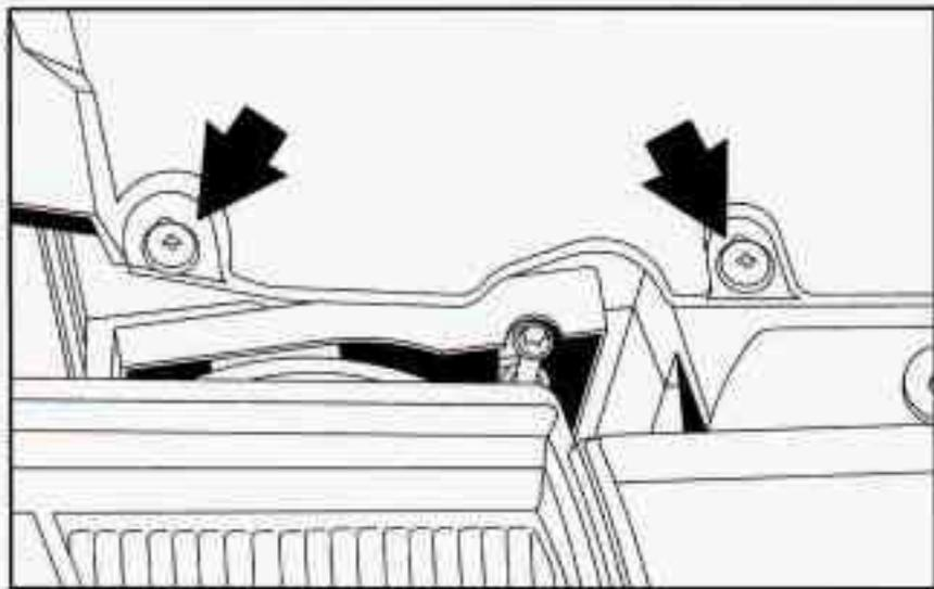
1. Remove the pins from the cover above the fog lamps.
