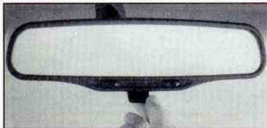
To reduce glare from lamps behind you, move the lever to the night position.
