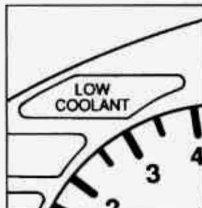
If this light comes on, your system is low on coolant and the engine may overheat. See "Engine Coolant" in the Index and have your vehicle serviced as soon as you can.
