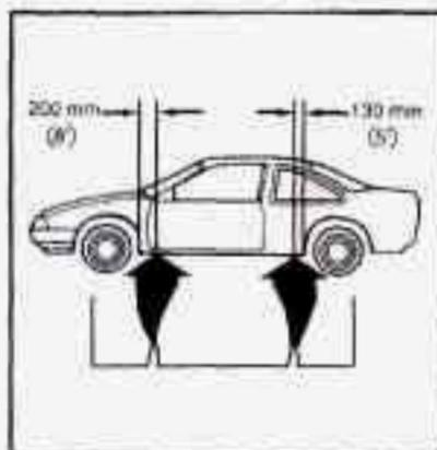
Position the jack under the vehicle and raise the jack lift head until it fits firmly into the notch in the vehicle's frame nearest the flat tire.
