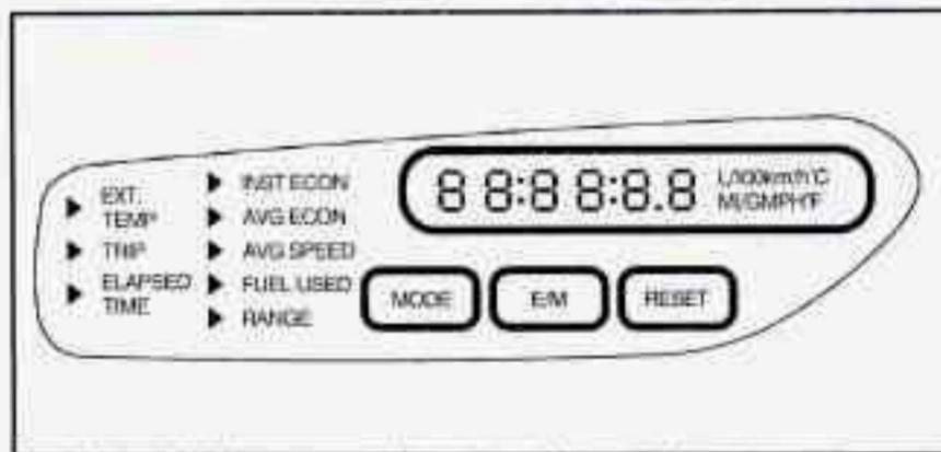
When you start your engine, the trip calculator will display a mode. A lighted arrow shows which mode is displayed.
