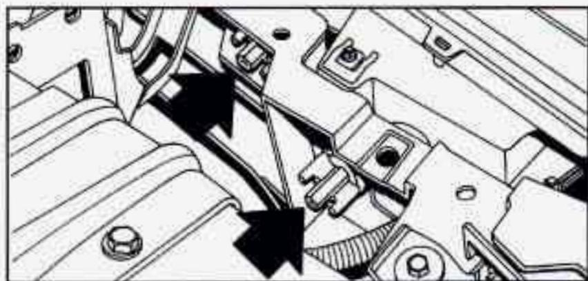
4. Remove the two wing nuts from the lamp bar on the passenger side.
