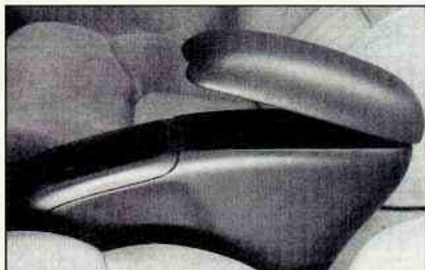
To open the storage area, press the latch on the front edge and pull up. The console has a cupholder, cassette tape storage and a coinholder.
