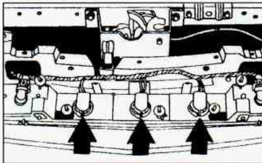
6. Squeeze the tab on the socket and turn the socket counterclockwise.
