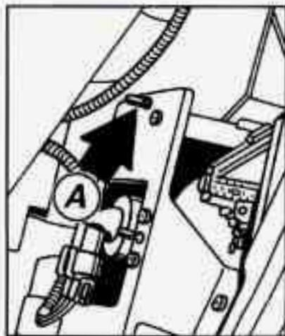
2. If the pointer isn't at 0 (zero), turn the horizontal aiming screw to adjust the aim.
