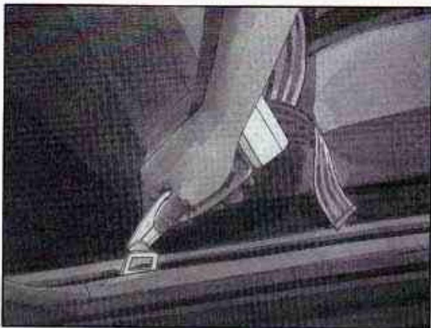
3. Put the belt's special latch plate into the vehicle's safety belt buckle.
