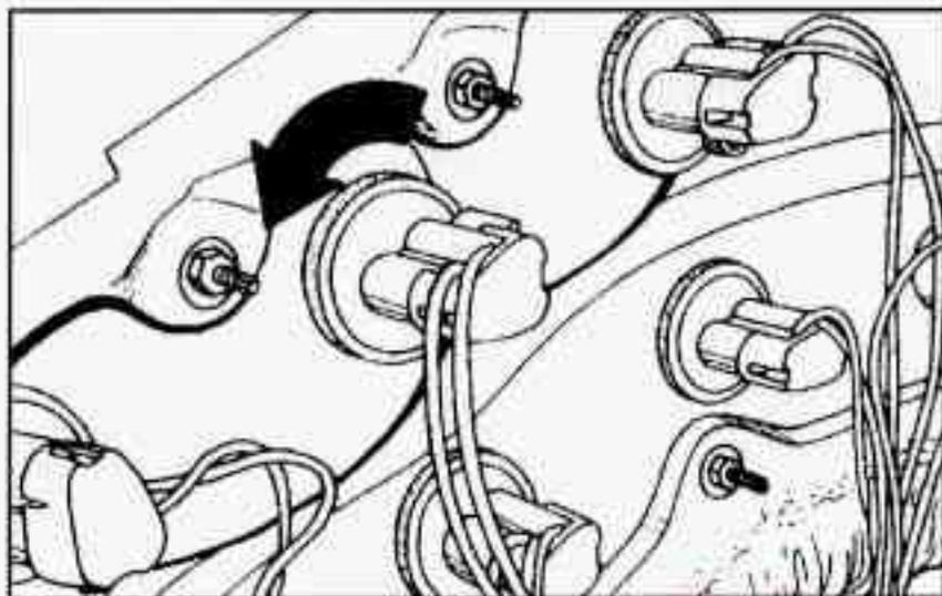
2. If the socket has a tab, squeeze it. Turn the socket counterclockwise.
