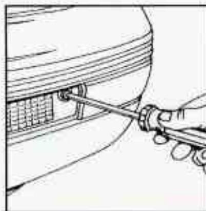
1. Remove the screws and pull the turn signal housing forward.
