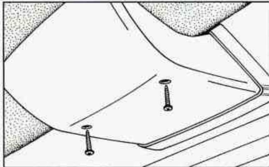
1. Remove the two screws from the cover.
