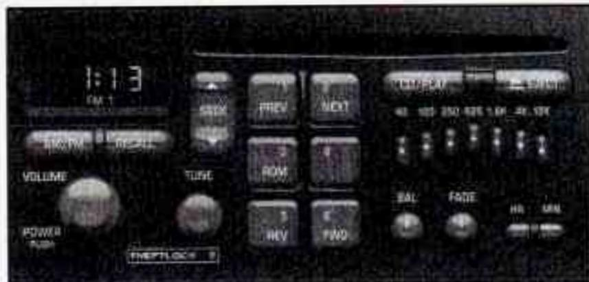
**RECALL:** Press this button to see which track is playing. Press it again within five seconds to see how long it has been playing (elapsed time). Press it again to return to time, or let the display return automatically.
