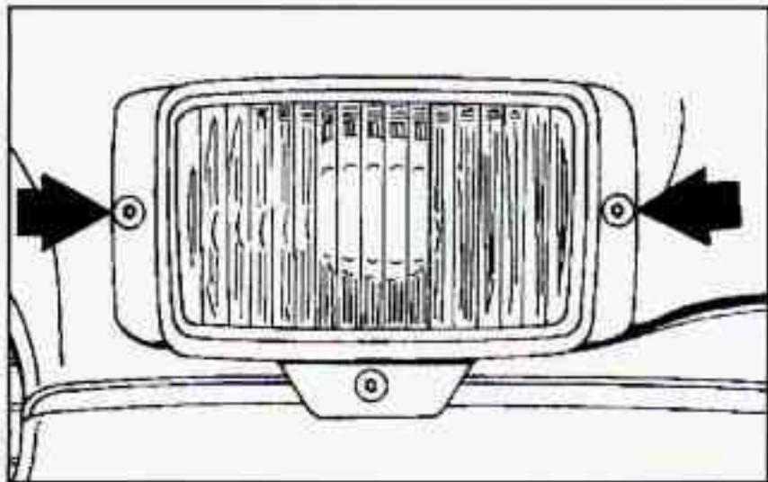
1. Remove the two screws and pull the housing away from the vehicle.
