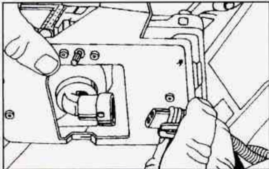
4. Lift the plastic locking tabs on the electrical connector and pull the connector from the headlamp socket.
