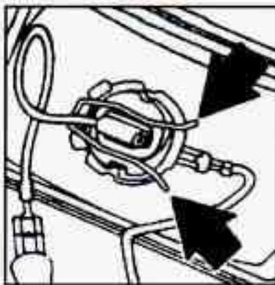
2. Remove the spring clip holding the bulb in the housing and pull out the bulb.
