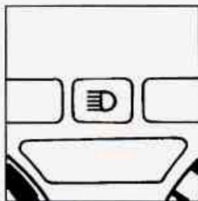
To change your headlamps from low beam to high beam, or high to low, pull the multifunction lever all the way toward you. Then release it. When the high beams are on, a blue light on the instrument panel also will be on.
