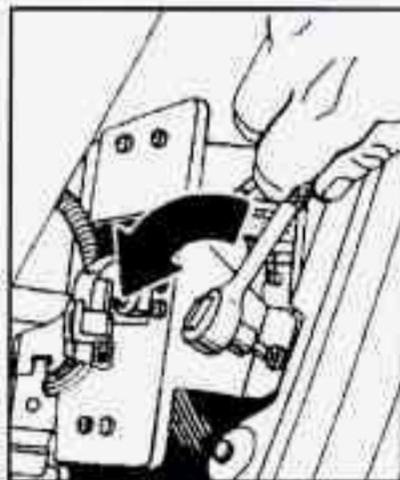
2. Remove the screw at the top of the headlamp support panel. Loosen the two screws at the bottom of the panel. Loosen these two screws until they are out of the headlamp frame, but still in the brackets on the headlamp assembly.
