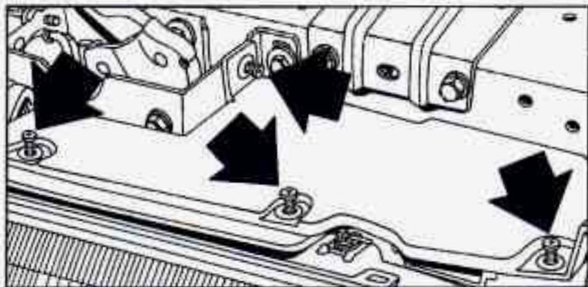
1. Remove the four pins from the cover on the driver side.
