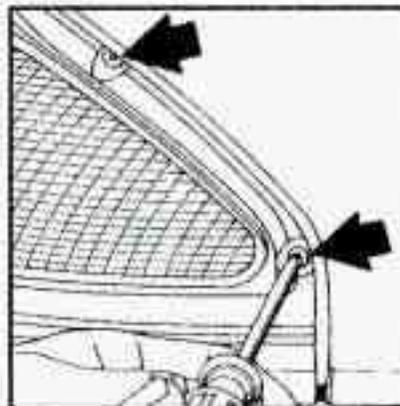
1. Remove the screws and pull the sidemarker housing forward.
