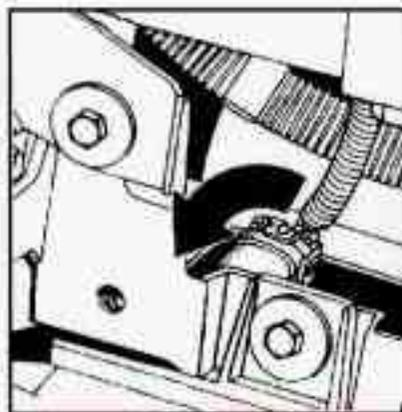
2. Turn the bulb socket counterclockwise until it pops loose from the housing.
