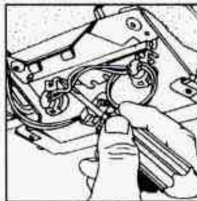
3. Lift the tabs at the top and bottom of the socket and pull it from the housing.
