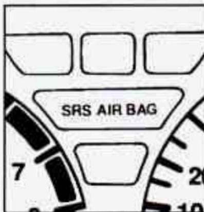
There is an air bag readiness light on the instrument panel, which shows SRS AIR BAG or the air bag symbol.
