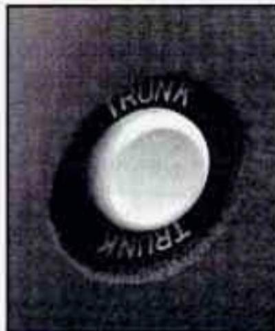
Press the button behind the glove box door to unlock the trunk from inside your vehicle. Your transaxle shift lever must be in PARK (P).
