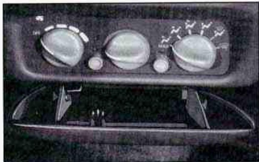
For the instrument panel ashtray, open it, push down on the locking tab and pull out the ashtray.
