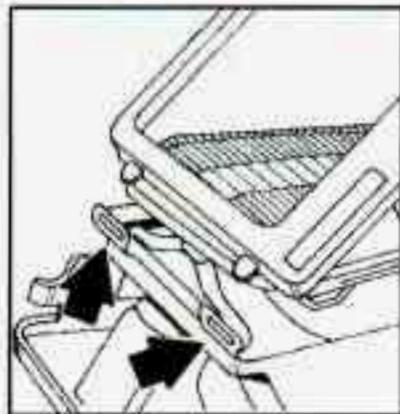
10. Insert the tabs on the aiming ring into the slots in the headlamp assembly.
