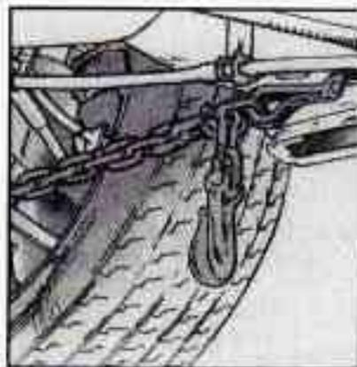
Attach T-hook chains into the slotted holes in the bottom of the floor pan support rails just ahead of the rear wheels on both sides.
