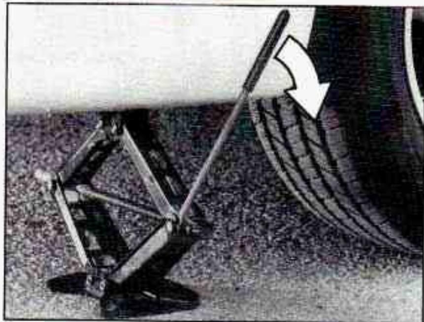
Raise the vehicle by turning the jack handle clockwise. Raise the vehicle far enough off the ground for the spare tire to fit under the vehicle. Remove all wheel nuts and take off the flat tire.
