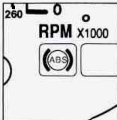
With the anti-lock brake system, this light will come on when you start your engine and it will stay on for three seconds. That's normal. If the light doesn't come on, have it fixed so it will be ready to warn you if there is a problem.
