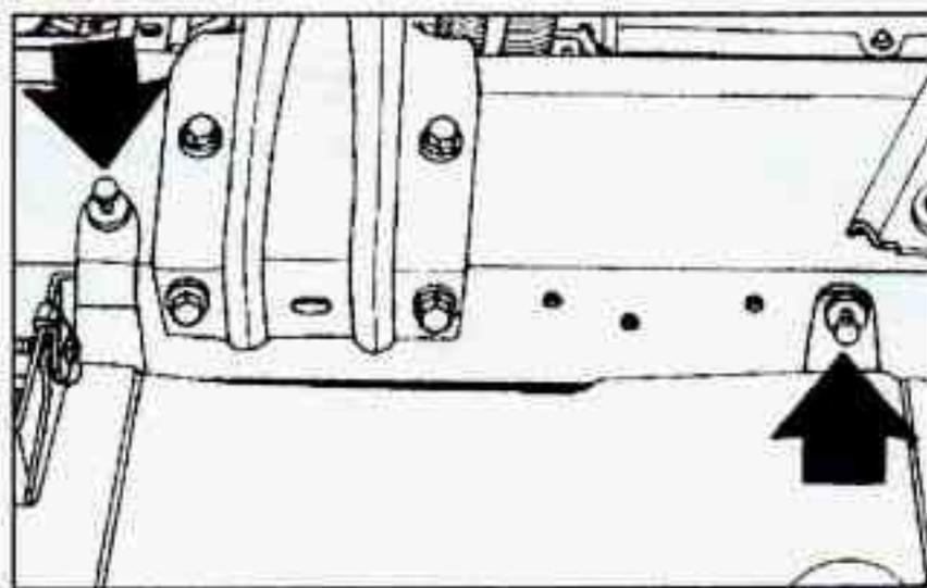
1. Remove the pins from the cover above the turn signal lamps.
