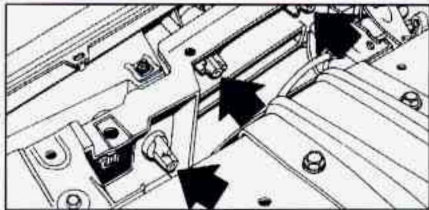
3. Remove the three wing nuts from the lamp bar on the driver side.
