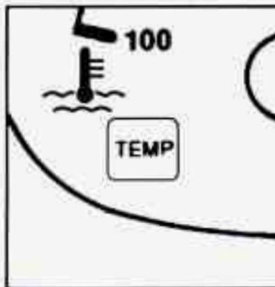
This light tells you that your engine coolant has overheated or your radiator cooling fan is not working.
