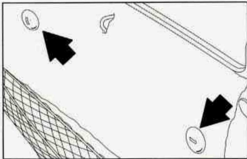
1. Remove the plastic retainers and pull the carpet away from the rear of the trunk.
