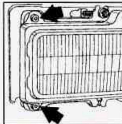
6. Remove the Torx® screws at the end of the aiming ring. The aiming ring will swing open like a gate.
