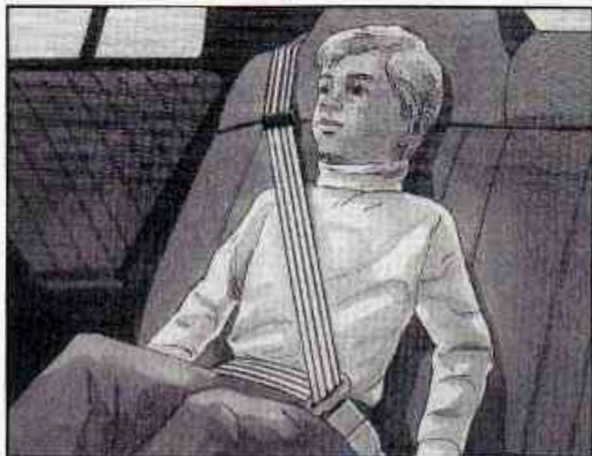
4. Buckle the belt around the child, and make sure that both the lap belt and the shoulder belt are secured properly. Make sure that the shoulder belt crosses the shoulder. See "Safety Belts, Rear Seat Passengers" in the Index.
