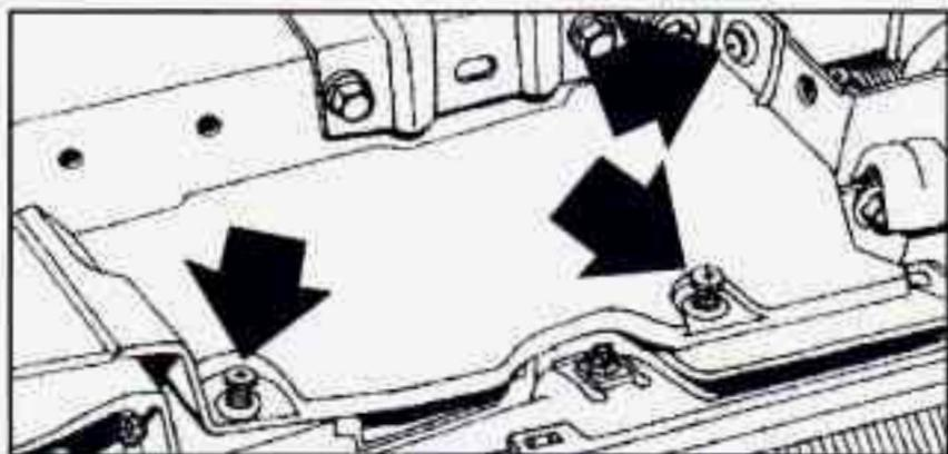
2. Remove the three pins from the cover on the passenger side.
