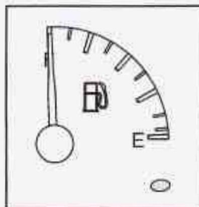
Your fuel gage tells you about how much fuel you have left, when the ignition is on. When the indicator nears EMPTY (E), you still have a little fuel left, but you should get more soon. An amber light will come on below the gage when the fuel tank is near EMPTY (E).
