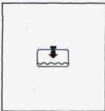
If this light comes on and stays on, the vehicle should be promptly pulled off the road and the coolant level checked. See "Engine Coolant" in the Index.
