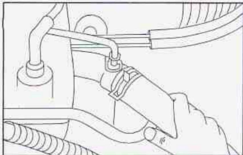
4. With the coolant surge tank pressure cap off, start the engine and let it run until you can feel the upper radiator hose getting hot. Watch out for the engine fan.
