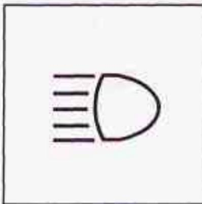
To change the headlamps from low beam to high or high to low, pull the turn signal lever all the way toward you. Then release it. When the **high** beams are on, this blue light on the instrument panel also will be on.
