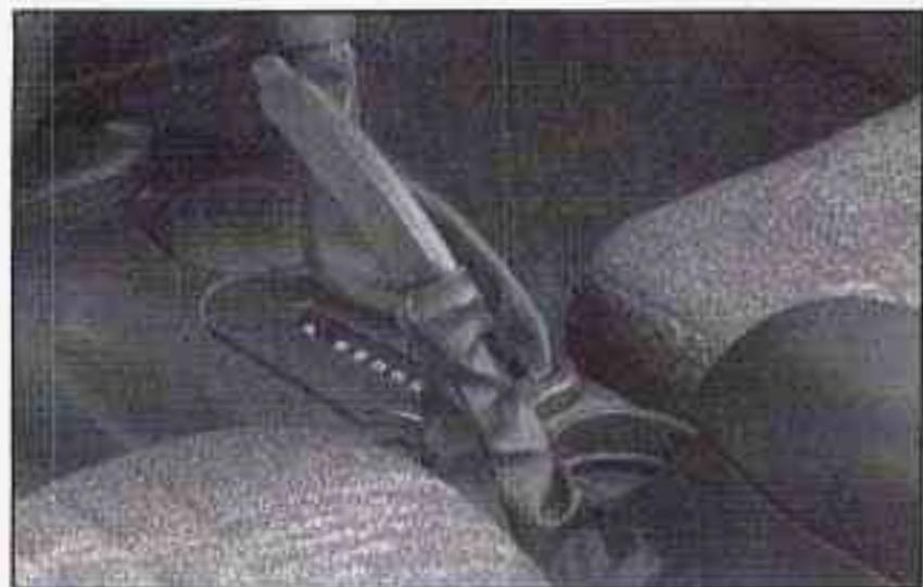
To set the parking brake hold the regular brake pedal down with your right foot. Pull up on the parking brake
