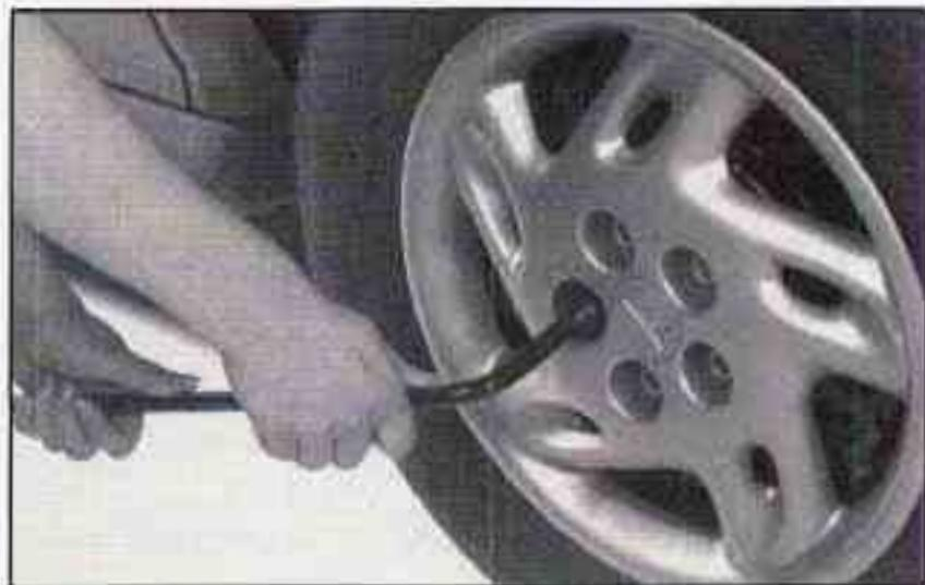
1. Remove the wheel nut caps (you may need to use the wheel wrench to loosen and remove them, if your fingers do not fit into this small area).
