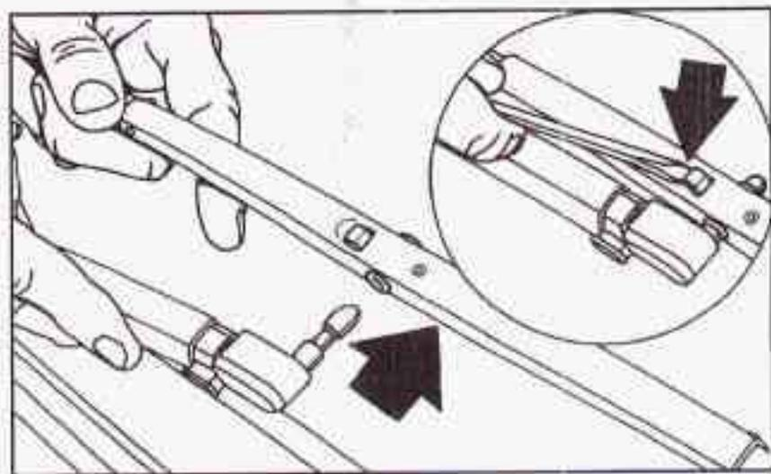
Replacement blades come in different types and are removed in different ways. Here's how to remove the type with a release clip:
