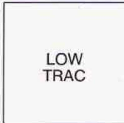
This light will come on when your Enhanced Traction System is limiting wheel spin. See "Enhanced Traction System Active Light" in the Index. You may feel or hear the system working, but this is normal.
