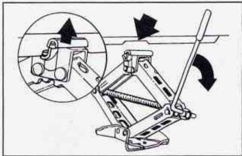
4. Raise the vehicle by rotating the wheel wrench clockwise. Raise the vehicle far enough off the ground so there is enough room for the spare tire to fit.
