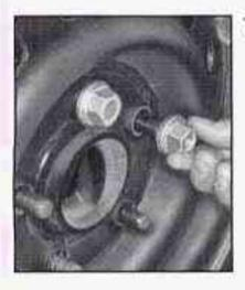
Replace the wheel nuts with rounded end of the nuts toward the wheel.
