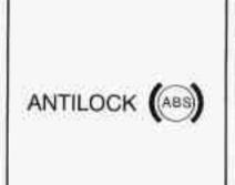
If there's a problem with the anti-lock brake system, this warning light will stay on. See "Anti-Lock Brake System Warning Light" in the Index.
