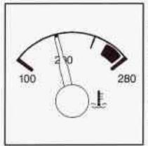
This gage shows the engine coolant temperature.
