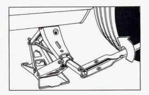
Lower the vehicle by rotating the wheel wrench counterclockwise on the jack. Lower the jack completely.
