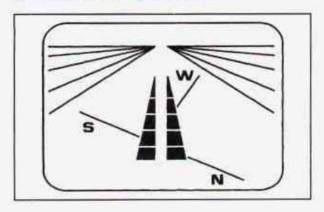
Some vehicles are equipped with an electronic compass. As with all compasses, this unit senses the earth's magnetic field to show the direction the car is pointing. The earth's magnetic field is not always the same direction as true north as we know it. So, you must enter a zone number to tell the compass the difference between magnetic and actual north. This tells the compass where in the country you are driving
