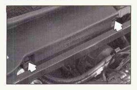
To check the fuses in this underhood fuse center, turn the two knobs one-quarter turn counterclockwise and loosen the metal wing nut on the passenger side of the cover. Then remove the cover. The inside of the cover has a chart that explains the features and controls governed by each fuse and relay.
