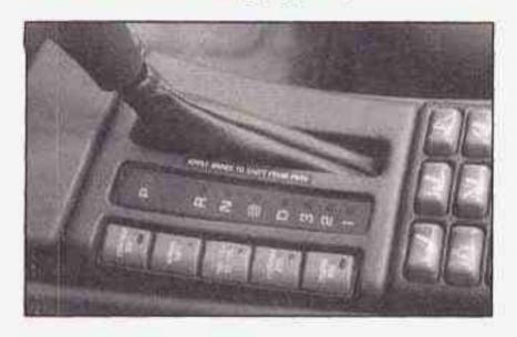
Press PERFORM SHIFT to allow the transaxle to shift at higher engine speeds, increasing acceleration performance. An indicator light on the switch will glow when performance shifting is in operation.
