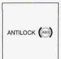
With the anti-lock brake system, the light(s) will come on when you start your engine and may stay on for several seconds. That's normal.
