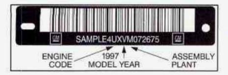
This is the legal identifier for your Pontiac. It appears on a plate in the front corner of the instrument panel, on the driver's side. You can see it if you look through the windshield from outside your vehicle. The VIN also appears on the Vehicle Certification and Service Parts labels and the certificates of title and registration.
