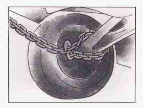
Attach a separate safety chain around the outboard end of each control arm.
