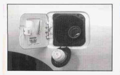
If you have the (L36) 3800 V6 engine, your fuel cap will be tethered and you cannot hang it on the inside fuel door while refueling.
