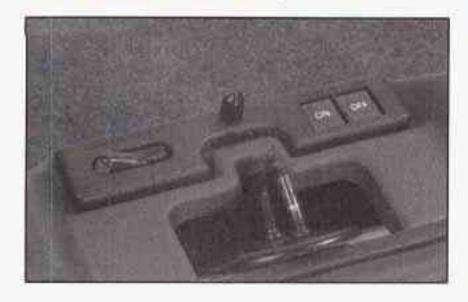
Some vehicles have an air inflator for use in maintaining proper air pressure for the tires. The air inflator is located in the trunk. The ON switch will work only with the ignition on.
