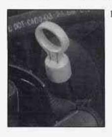
The transaxle fluid dipstick top is a round, red loop and is next to the brake master cylinder behind the engine block. Pull out the dipstick and wipe it with a clean rag or paper towel.
