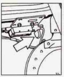
If your vehicle has a fuel door lock, the fuel door can be opened manually in case of an electrical power failure.
