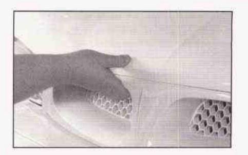
Then go to the front of the vehicle and push up on the secondary hood release.
