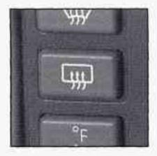
The lines you see on the rear window warm the glass. Press the button to start warming your window, If you have the standard system, a light will glow in the switch while the defogger is working. After 10 minutes it will turn off by itself or press the button during the heating cycle to turn it off. If you need additional warming time, push the button again. The system will then operate for five minutes before going off by itself.
