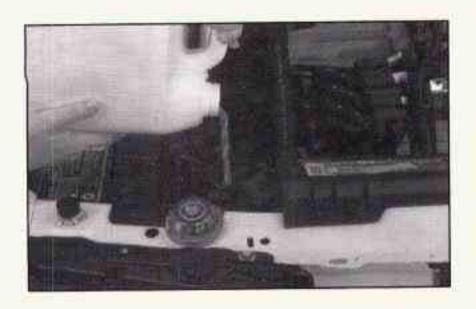
Fill the radiator with the proper DEX-COOL<sup>®</sup>
