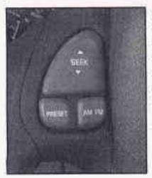
SEEK: Press the up arrow to tune to the next radio station and the down arrow to tune to the previous radio station. If a cassette tape or compact disc is playing, the player will advance with the up arrow and rewind with the down arrow.
