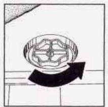
The equipment you'll need is in the trunk. Pull the carpeting from the floor of the trunk. Turn the center retainer bolt on the spare tire cover counterclockwise to remove it.
