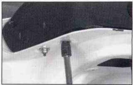
Remove the five nuts that hold the assembly in place with a 10 mm socket. Pull the carpet up and out of the way to remove the center nut. (There are two nuts on the driver's side, two on the passenger's side and one in the middle.)
