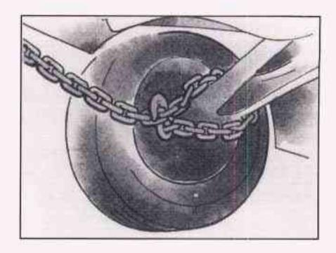
Attach a separate safety chain around the outboard end of each lower control arm.
