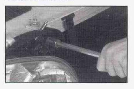
1. Remove the two bolts with a 10 mm socket.
