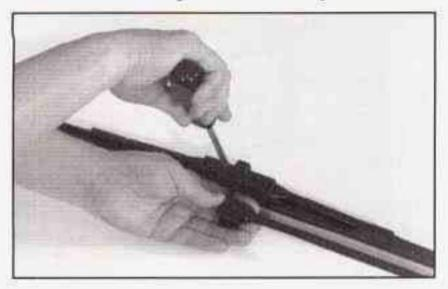
Replacement blades come in different types and are removed in different ways. Here's how to remove the type with a release clip:
