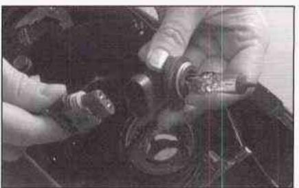
Replace the bulb and reverse the steps to install the new bulb assembly.
