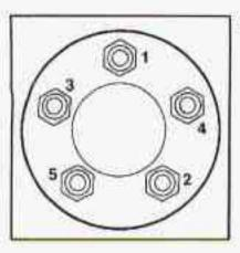
Tighten the wheel nuts firmly in a criss-cross sequence.
