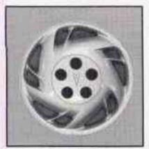
To remove the wheel or nut cap covers for your particular vehicle, if you have steel wheels with full plastic wheel covers, loosen each nut cap using the wheel wrench.
