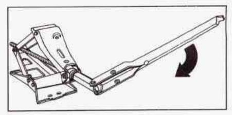
Attach the wheel wrench to the jack, and rotate the wrench clockwise to raise the jack head a few inches.
