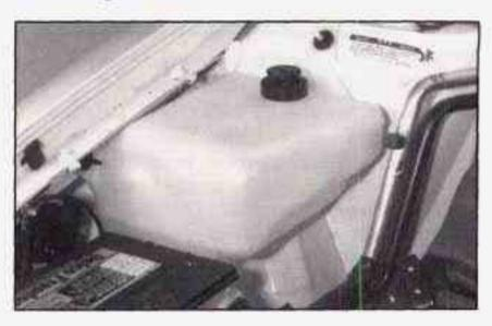
When your engine is cold, the coolant level should be at FULL COLD or a little higher. When your engine is warm, the level should be up to FULL HOT or a little higher.
