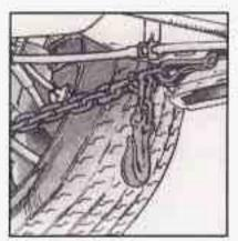
Attach T-hook chains to slots in the bottom of the floor pan directly ahead of rear wheels on both sides.
