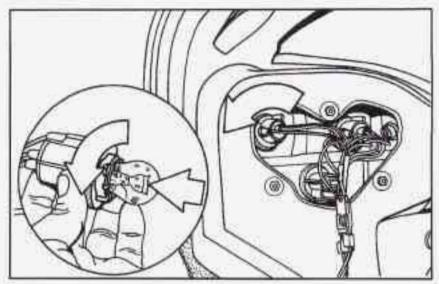
Turn the bulb socket assembly counterclockwise to remove it from the lamp assembly.
