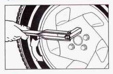
Use the wheel wrench to loosen the wheel nuts, but don't remove them.
