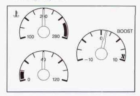
Vehicles equipped with the supercharged engine have this boost gage that indicates vacuum during light to moderate throttle and boost under heavier throttle. The gage displays the air pressure level in psi going into the engine's combustion chamber.
