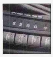
To turn the system off, press the TRACTION CONTROL button located on the console next to the gear shift selector.
