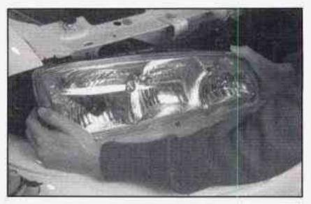
Slide the headlamp assembly outward (to the left) and lift it out.
