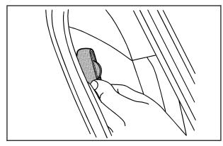
Pull the elastic cord out from between the edge of the seatback and the interior body to remove the guide from its storage clip.
