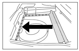
2. The trunk cargo cover must be fully closed, and the trunk must be closed before raising the hardtop.
