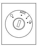
With the key in the ignition switch, you can turn it to four different positions.
