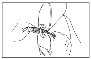
If your seat has a safety belt guide, and the safety belt is not routed through the guide, slide the edge of the belt webbing through the opening on the guide. Be sure the belt is not twisted. 3. Pick up the latch plate and pull the belt across you. Do not let it get twisted.
