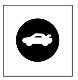
Press this button located on the driver's door near the map pocket to open the trunk.
