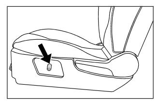
To adjust a power lift seat, press the top or bottom of the power lift seat switch to raise or lower the seat.
