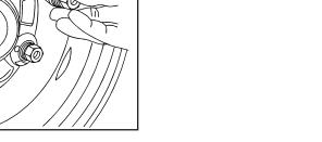
10. Remove any rust or dirt from the wheel bolts, mounting surfaces, and spare wheel.
