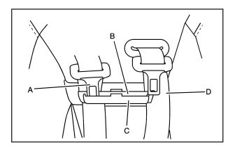
If your vehicle has a retractable hardtop, secure the safety belt latch plate when the safety belt is not in use in the rear seat. To do this, slide the safety belt webbing (D) behind the belt webbing retaining clip (B) and slide the latch (A) into the latch retaining clip (C).
