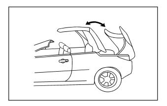
As the switch is being pressed the windows and trunk lid will open. The hardtop will automatically lower into the trunk, and the trunk lid will close and latch. If the engine is on, a chime will sound when the hardtop has lowered completely. The Driver Information Center (DIC) will display TOP MOVE COMPLT to signal the procedure is complete. See *DIC Warnings and Messages on page 3-46* for more information.
