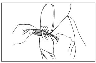
Remove the safety belt from the headrest-mounted guide.
