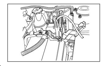
6. Connect the red positive (+) cable to the positive (+) terminal of the dead battery.
