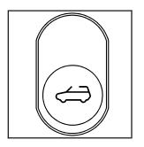
4. The hardtop switch is located on the headliner between the front reading lamps. Press and hold the switch forward to raise the hardtop. The switch must be pressed until the cycle is complete.
