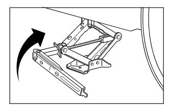
Raise the vehicle by turning the wheel wrench clockwise. Raise the vehicle far enough off the ground so there is enough room for the compact spare tire to fit underneath the wheel well.
