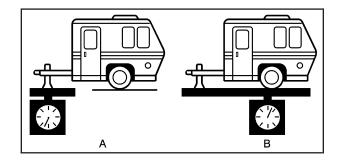
If you are using a weight-carrying hitch, the trailer tongue (A) should weigh 10 to 15 percent of the total loaded trailer weight (B).
