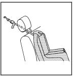
If the position you are using has a headrest or head restraint and you are using a single tether, route the tether under the headrest or head restraint and in between the headrest or head restraint posts.
