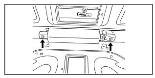
Remove the cover by pressing the tabs at either end with a tool.
