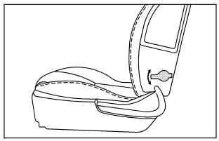
If your vehicle has this feature, the handle is located on the outboard side of the driver's seat. Move the handle up repeatedly to decrease lumbar support. Move the handle down repeatedly to increase lumbar support.
