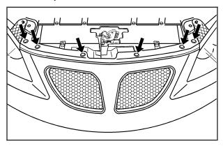
Loosen the front fascia by removing the plastic push pins along the top of the tie bar by prying under the fasteners with a tool. Pull back the front fascia then pull the headlamp assembly forward, out of the vehicle. You need to pry the headlamp assembly away from the fender. This frees the ball stud from its retainer in the fender bracket.
