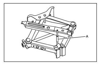
Place the jack over the bolt (A) on the floor, making sure it contacts the bolt as shown, and thread the jack retainer nut until it contacts the jack.
