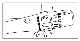
Use this lever, located on the right side of the steering wheel, to operate the windshield wipers.
