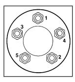
Tighten the wheel nuts firmly in a crisscross sequence, as shown, with the wheel wrench.
