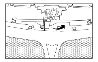
2. Then go to the front of the vehicle and push the secondary hood release lever to the right.
