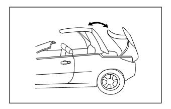
As the switch is being pressed the hardtop will raise from the trunk and move into place. The hardtop and trunk lid will close and latch. If the engine is on, a chime will sound when the hardtop has raised completely. The Driver Information Center (DIC) will display the TOP MOVE COMPLT message to signal the procedure is complete. See *DIC Warnings and Messages on page 3-46* for more information.
