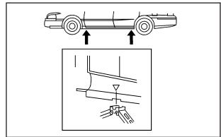
5. Position the lift head at the jack location nearest the flat tire. Make sure all of the jack lift head is touching the jacking flange under the body. Do not place the jack under a body panel. The lower body panel has an arrow to aid in locating the jacking location. Put the compact spare tire near the flat tire being changed.
