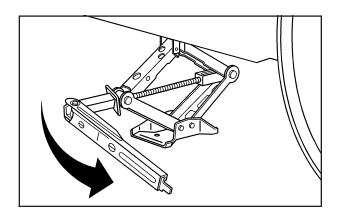
Lower the vehicle by turning the wheel wrench counterclockwise. Lower the jack completely.
