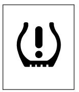
When a low tire pressure condition is detected, the TPMS turns on the low tire pressure warning light located on the instrument panel cluster.
