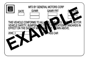
A vehicle specific Certification label, found on the rear edge of the driver's door, tells you the gross weight capacity of your vehicle, called the Gross Vehicle Weight Rating (GVWR). The GVWR includes the weight of the vehicle, all occupants, fuel and cargo. Never exceed the GVWR for your vehicle, or the Gross Axle Weight Rating (GAWR) for either the front or rear axle.
