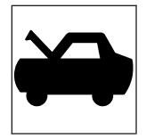
Pull the handle with this symbol on it. It is located under the instrument panel on the driver's side of the vehicle.
