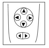
The controls for the outside power mirrors, are located on the driver's door.
