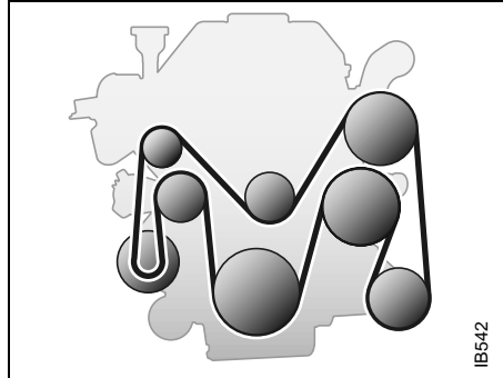
Routing of the Poly-Vee-belt: 4-cylinder engine with A/C
