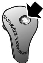
To select **Sport mode**, press the "S" button on the selector lever when the selector lever is in position N, D, 3, 2 or 1.
