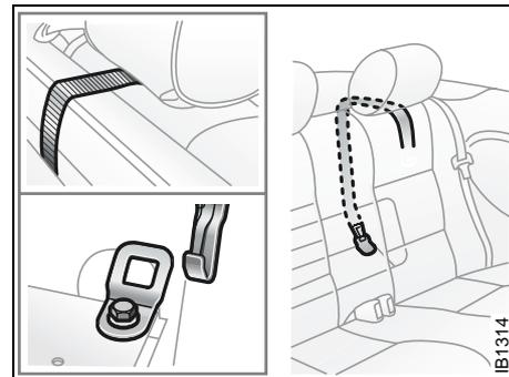
*Attaching tether strap hook to anchorage, Convertible.
