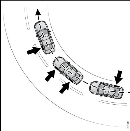
*Illustration of how the system applies the brakes on one or several wheels to avoid a skid*
