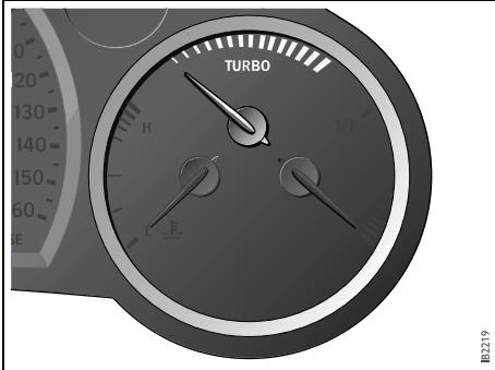
If the needle repeatedly enters the red zone and the engine at the same time loses power, because the monitoring system is limiting the boost pressure, you should contact a Saab dealer as soon as possible. When the speed of the car exceeds 143 mph (230 km/h), acceleration is limited by reducing the boost pressure. The pressure gauge then moves towards the middle of the white field, indicating a drop in engine power and consequently the car's speed.
