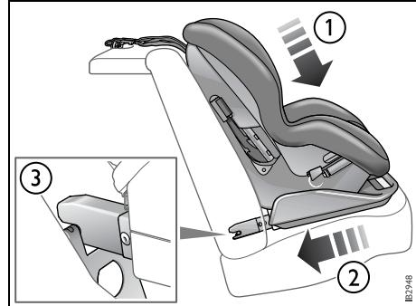
*Rigid 2-point lower anchorage with top tether*
