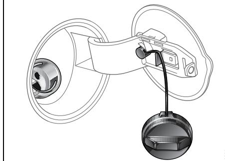
*Filler cap removed for refueling*
