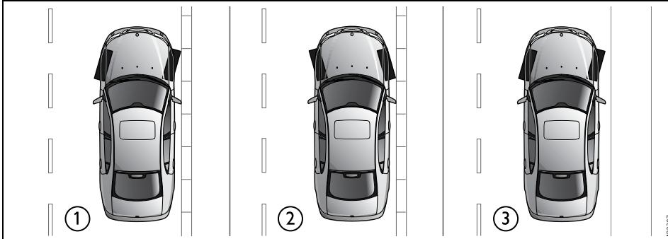
**1 Downhill with curb.** Turn the wheels toward the curb and edge the car forwards until the wheel lightly touches the curb.
