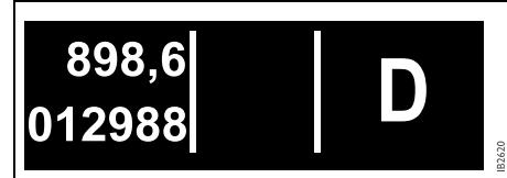
*Indication of gear position on main instrument panel*
