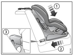
Rigid 2-point lower anchorage with top tether
