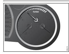
If the needle repeatedly enters the red zone and the engine at the same time loses power, because the monitoring system is limiting the boost pressure, you should contact a Saab dealer as soon as possible. When the speed of the car exceeds 143 mph (230 km/h), acceleration is limited by reducing the boost pressure. The pressure gauge then moves towards the middle of the white field, indicating a drop in engine power and consequently the car's speed.
