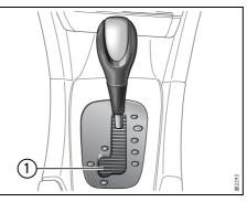
Selector lever 1 Position for manual gear selection
