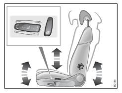
Adjust the height of the seat with the rear
