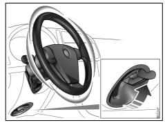
Lever for steering wheel adjustment
