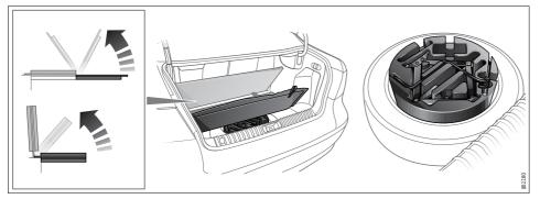
The spare wheel, the tools and the jack with its crank are carried under a panel in the trunk.
