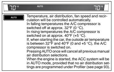
AC The A/C compressor must be turned on and off manually with the AC button. The compressor can only be turned on or off while the engine is running. This function has two modes: • AC – The system cools and dehumidifies the incoming air. This symbol is not shown in the display. • AC-OFF – The A/C compressor is switched off. The incoming air is not cooled or dehumidified. See also Profiler on page 93.
