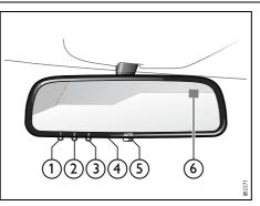
Buttons for garage opener, autodimming and compass
