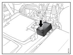
Battery disconnect switch with reset button
