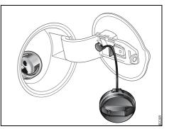
Filler cap removed for refueling
