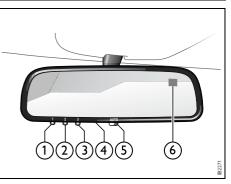
Buttons for garage opener, autodimming and compass
