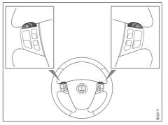
Steering wheel controls for manual gear selection (Vector models)
