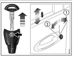
Locking/unlocking the front left-hand door with the traditional key 1 Lock
