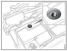
Checking the battery electrolyte level. Level correct if level indicator dark
