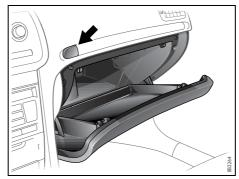
Open the glove compartment with the button on the left of the moulding
