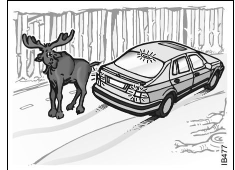
Braking with ABS – evasive steering
