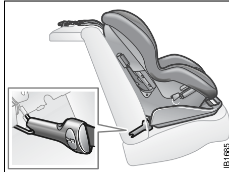
Semi-rigid 2-point lower attachment with top tether
