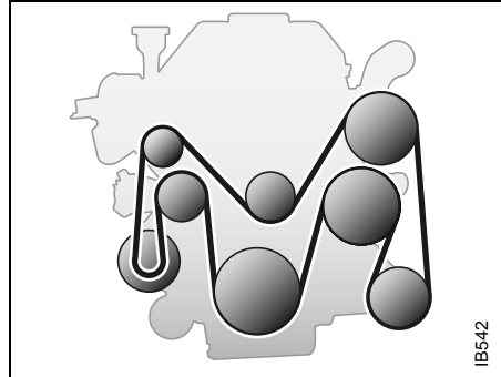
Routing of the Poly-V-belt: 4-cylinder engine
