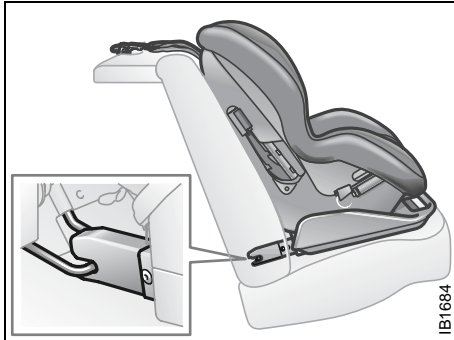
Rigid 2-point lower attachment with top tether
