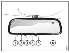
Buttons for garage opener, autodimming and compass
