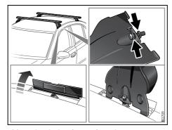
Mounting holes for roof carrier
