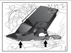
Turn the two retainers a quarter turn to unlock the battery cover.
