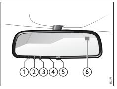
Buttons for garage opener, autodimming and compass
