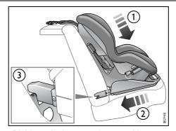
Rigid 2-point lower anchorage with top tether
