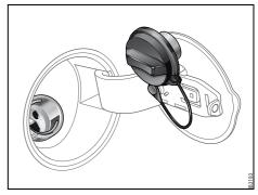
Filler cap removed for refueling
