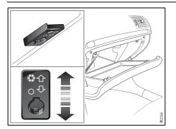
Sliding cover in glove compartment to admit cold air (cars with ACC only). This allows the storage of chocolate and chilled drinks, for example.
