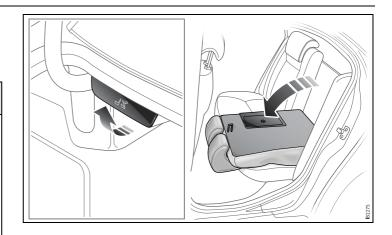
For greater flexibility, the rear seat is split so that the narrow and the wide part can be folded down separately.
