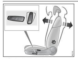
Adjusting the rake angle
