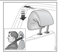
Therefore, the SAHR does not normally need to be replaced or repaired after a rearend crash.
