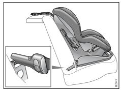
Semi-rigid 2-point lower anchorage with top tether
