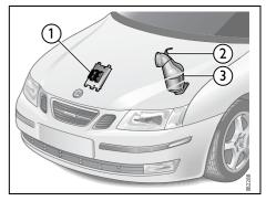
Engine management system with catalytic converter
