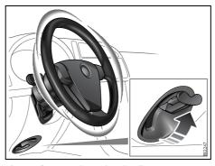
Lever for steering wheel adjustment
