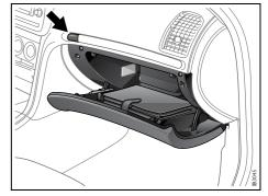
Open the glove compartment with the button on the left of the moulding. Convertible has lockable glove compartment. Use the traditionally key, see page 46.
