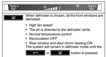
The following three buttons for air distribution can be selected individually or in combination. Press the button or selection of buttons to produce the airflow you desire. Pressing the same button twice will return the system to AUTO. You can also select automatic air distribution by pressing the AUTO button.
