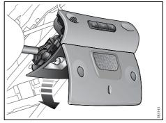
Hatch opened for replacement of center bulb
