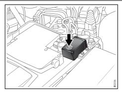
Battery disconnect switch with reset button
