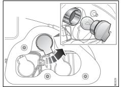
If a brake light bulb fails, the adjacent taillight will act as a brake light to ensure traffic safety. Change the broken bulb when possible.
