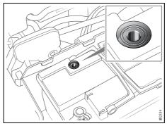
Checking the battery electrolyte level. Level correct if level indicator dark. Battery should be changed if indicator is light
