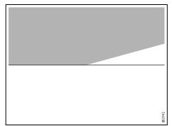
Correctly adjusted low beam
