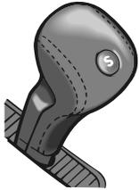
To select Sport mode, press the "S" button on the selector lever when the selector lever is in position N or D.
