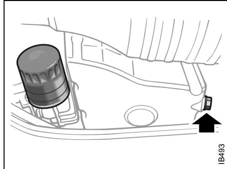
*Drain plug and oil filter*
