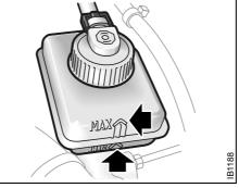
Brake and clutch-fluid reservoir
