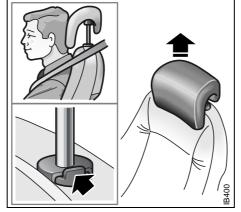
The head restraint can be raised or lowered and is adjustable in various positions.
