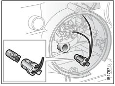
Parking-light bulb (cars with halogen low beam)
