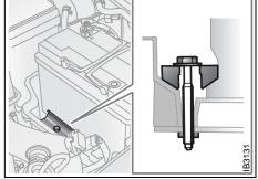
Correct position for battery clamp
