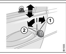
Locking/unlocking by key 1 To lock 2 To unlock
