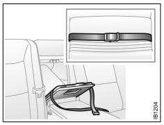
Fitting the locking strap on the center armrest, Saab 9-5 Sedan (not needed on SportWagon). The locking strap is standard equipment in
