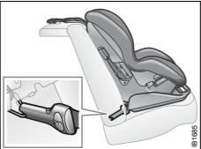
Semi-rigid 2-point lower attachment with top tether
