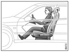
Correctly positioned safety belt
