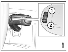
Control for setting wiper delay 1 Long delay 2 Short delay
