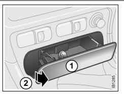
Front ashtray 1 Press soft to open/close 2 Pull out one side at an angle
