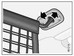
Attaching the cargo net to the roof
