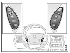
Audio System controls on steering wheel
