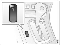
Switch for operation of central locking
