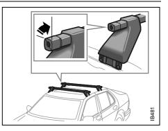
3 Start on the left-hand side of the car. Rest the carrier carefully across the roof, with the rigid foot towards you. Hold the foot clear of the roof to avoid damaging the paintwork.
