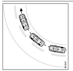
Increased stability with ESP. The system applies the brakes to the wheels as shown to prevent the car from skidding
