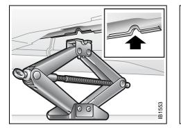
The collapsible jack handle is stowed in a cloth bag by the spare wheel. With the help of your foot, extend the handle as illustrated
