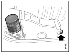
Drain plug and oil filter
