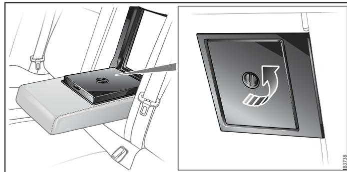
A load-through hatch is incorporated in the rear seat backrest to enable long, narrow items to be carried inside the car.
