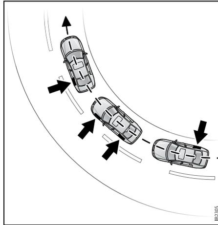
*Illustration of how the system applies the brakes on one or several wheels in order to reduce the likelihood of the car skidding*
