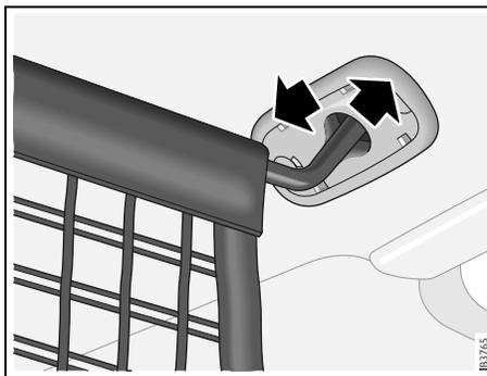
*Attaching the cargo net to the roof*
