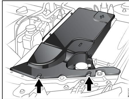
*Turn the two retainers a quarter turn to unlock the battery cover.*
