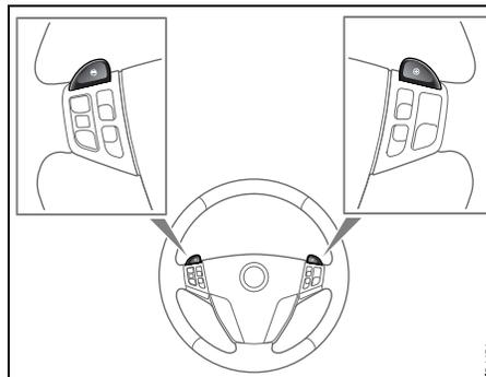
*Steering wheel controls for manual gear selection \**
