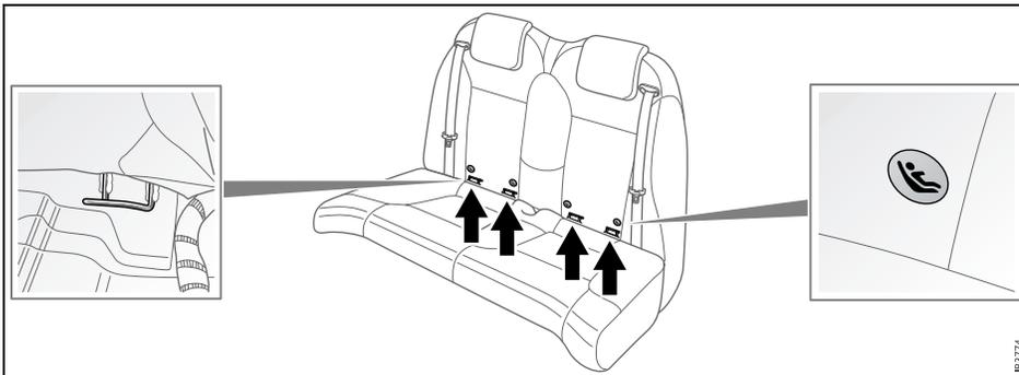
(Lower Anchor): Seating positions with two lower anchors.
