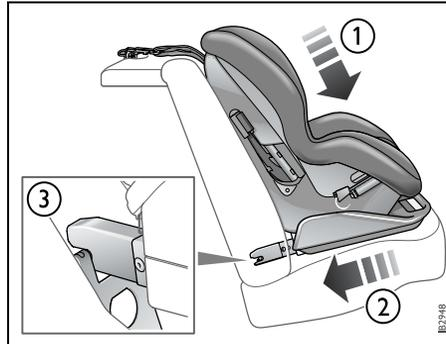
*Rigid 2-point lower anchorage with top tether*
