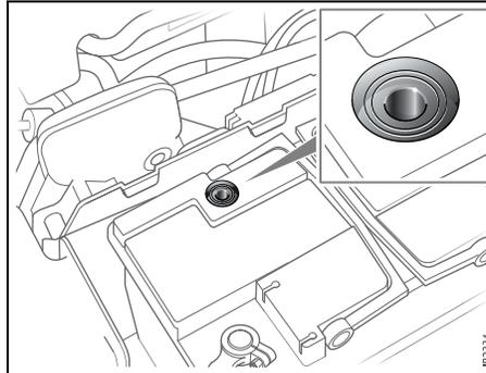
*Checking the battery electrolyte level.
