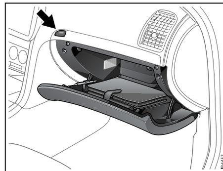
*Open the glove box with the button on the left of the moulding.
