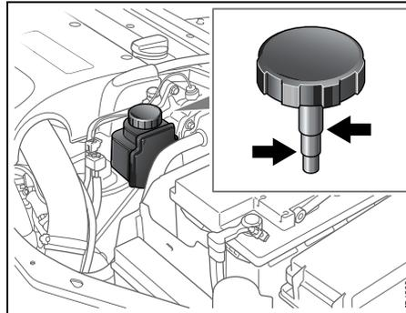
*Power steering fluid reservoir, 4-cyl engine*
