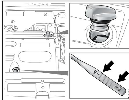
*Oil filler cap and dipstick, 4-cyl engine*
