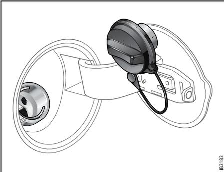
*When refueling, hang the filler cap inside the fuel door*
