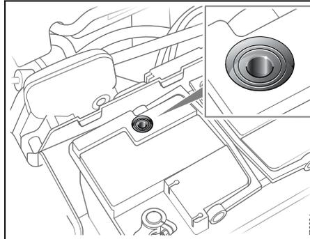
*Checking the battery electrolyte level.
