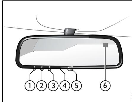
*Buttons for garage opener, autodimming and compass*
