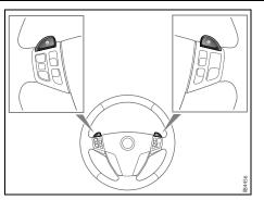
Steering wheel controls for manual gear selection \*
