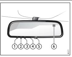
Buttons for garage opener, autodimming and compass
