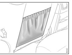
Sliding cover in glove box to admit cold air \*. This allows the storage of chocolate during hot weather for example.
