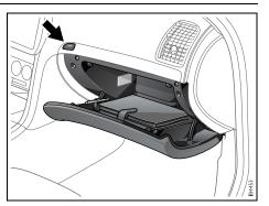
Open the glove box with the button on the left of the moulding. Convertible has lockable glove box. Use the traditionally key, see page 54.
