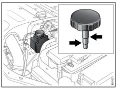
Power steering fluid reservoir, 4-cyl engine
