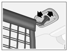
Attaching the cargo net to the roof
