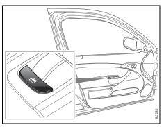
Button for temporary deactivation of rear door window switches and temporary override of window pinch protection
