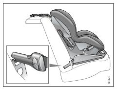
Semi-rigid 2-point lower anchorage with top tether
