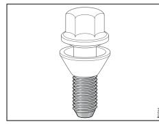
Grease the surfaces indicated with a thin layer of grease
