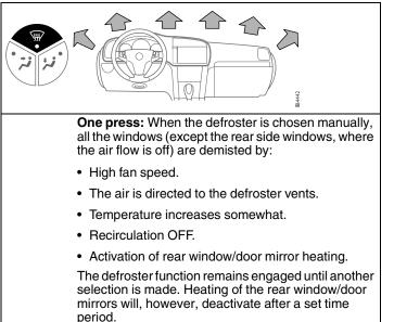
Two presses: Air is directed to the windscreen without the fan speed being increase or the rear window heating being switched on.
