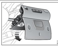
Hatch opened for replacement of centre bulb
