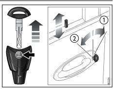
Locking/unlocking the front left-hand door with the traditional key 1 Lock 2 Unlock
