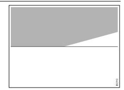
Correctly adjusted low beam
