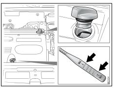
Oil filler cap and dipstick, 4-cyl engine
