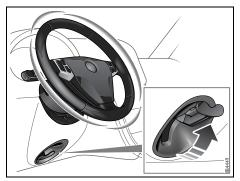
Lever for steering wheel adjustment
