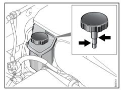
Power steering fluid reservoir, V6 engine
