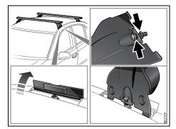
Mounting holes for roof carrier
