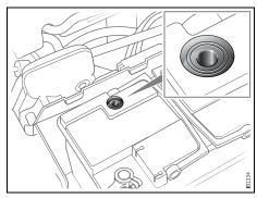
Checking the battery electrolyte level. Level correct if level indicator dark. Battery should be changed if indicator is light
