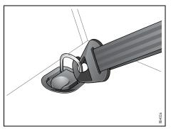
Cargo net fitted in front anchorage eye
