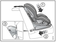
Rigid 2-point lower anchorage with top tether
