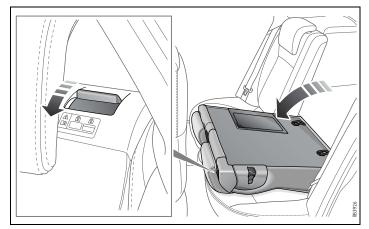
When returning the backrest to its upright position, make sure that it locks properly in place. The red indicator by the handle must not be visible. Also make sure that the seatbelt does not get caught.
