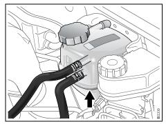
Coolant expansion tank, 4-cyl engine
