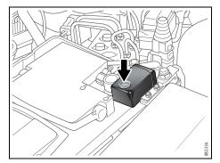
Battery disconnect switch with reset button
