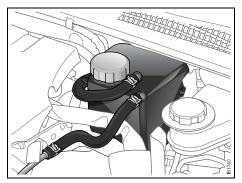
Coolant expansion tank, V6 engine
