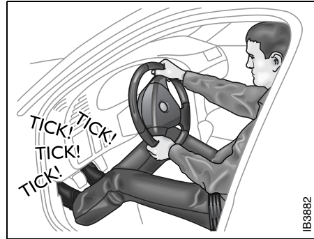
Braking with ABS brakes. When the system is operating, the brake pedal will pulsate gently and the system will make a ticking noise.
