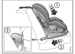
Rigid 2-point lower anchorage with top tether
