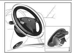
Lever for steering wheel adjustment
