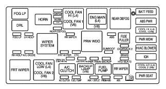
The underhood fuse block is located in the forward part of the engine compartment near the battery.
