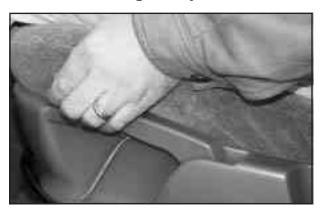
If your vehicle has a driver's seat height adjuster, it is located on the outboard side of the seat.
