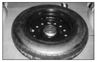
Vehicles equipped with the 3.5L V6 (L66) engine and aluminum wheels, must remove the center cap from the wheel prior to placing it on the load floor. To remove the center cap, tap the cap for the backside of the wheel, then place the wheel on the load floor.
