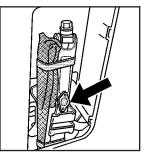
Install the jack in the driver's side panel of the rear cargo area and secure with the wingbolt.
