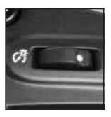
The thumbwheel for this feature is located on the instrument panel to the left of the steering column.
