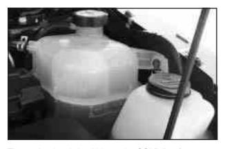
The coolant level should be at the COLD line (surge tank seam). If it is not, you may have a leak at the radiator hoses, heater hoses, radiator, water pump or somewhere else in the cooling system.
