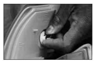
4. Rotate the side marker bulb socket counterclockwise and remove it from the housing.
