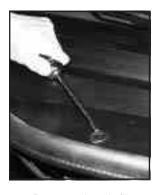
Remove the push pins from the air filter access panel.
