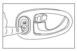
Press the bottom half of the switch on either front door to lock all of the doors. Push the top half of the switch to unlock all of the doors. The unlocked door indicators on the manual door lock pins will be hidden when the doors are locked.
