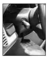
The lever that allows you to tilt the steering wheel is located on the left side of the steering column.
