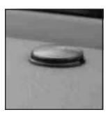
Your vehicle has a light sensor located on top of the instrument panel. Make sure it is not covered, or the headlamps will be on when you don't need them.
