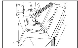
4. The safety belts in the rear outside seating positions have a child restraint locking feature. If you are using a rear outside seating position, pull the rest of the shoulder belt all the way out of the retractor to set the lock.
