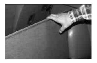
Lift the forward floor panel of the load floor cargo organizer.
