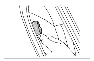
Pull the elastic cord out from between the edge of the seatback and the interior body to remove the guide from its storage clip.
