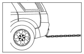
The recovery hook is located at the rear of your vehicle. It can only be used for pulling your vehicle out if it is stuck, not for towing the vehicle.
