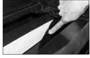
3. Remove the air filter from the housing by depressing the tab on the inboard side of the housing.
