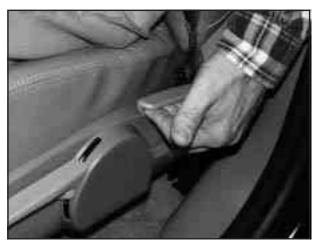
To adjust the seatback, lift the lever on the outboard side of the seat and move the seatback to where you want it. Then release the lever to lock the seatback in place.
