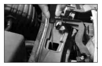
Insert a flat blade screwdriver through the opening in the top. Make sure the screwdriver fits through the opening in the headlamp bracket lower arm.
