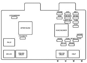
The instrument panel fuse block is located by the passenger's left leg.
