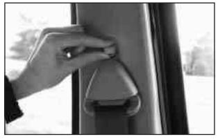
To move it down, squeeze the release button and move the height adjuster to the desired position. You can move the adjuster up just by pushing up on the shoulder belt guide. After you move the adjuster to where you want it, try to move it down without squeezing the release button to make sure it has locked into position.
