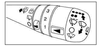
The lever on the right side of the steering column operates the windshield wipers.
