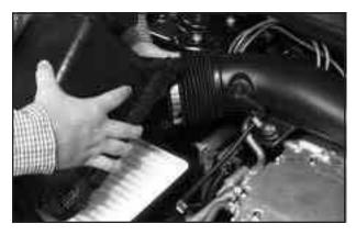
Remove air cleaner cover assembly and air filter element.
