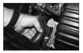
4. With the coolant surge tank pressure cap off, start the engine and let it run until you can feel the upper radiator hose getting hot. Watch out for the engine cooling fans. By this time, the coolant level inside the coolant surge tank may be lower. If the level is lower, add more of the proper DEX-COOL® coolant mixture to the coolant surge tank until the level reaches the COLD line.
