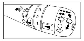
There is a band on the wiper lever to operate the rear wiper/washer.
