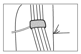
Be sure that the belt is not twisted and it lies flat. The elastic cord must be under the belt and the guide on top.
