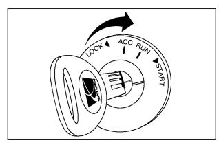
With the key in the ignition switch, you can turn it to four different positions.
