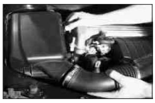
1. Unscrew the clamp on the air duct hose.
