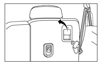
Lift the lever on the upper back corner of the seatback to move it to the desired position and then release it. Push and pull on the seatback to be sure it is locked in place.
