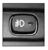
The button for your fog lamps is located in the instrument panel above the radio.
