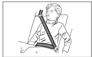
Buckle, position and release the safety belt as described in *Rear Seat Passengers on page 1-23*. Make sure that the shoulder belt crosses the shoulder.
