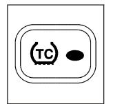
If your vehicle is equipped with the 2.2L four cylinder engine, the traction control system can be turned off by pressing the traction control button. It is located on the instrument panel above the audio system.
