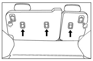
Anchor the top strap to one of the anchor points shown in the illustration. Be sure to use an anchor point located on the same side of the vehicle as the seating position where the child restraint will be placed. If you have an adjustable head restraint, raise the head restraint and route the top strap under it.
