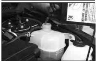
The vehicle must be on a level surface. When your engine is cold, the coolant level should be at the Cold line (surge tank seam). When your engine is warm, the level should be at the Cold line or a little higher.
