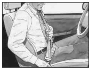
To make the lap part tight, pull down on the buckle end of the belt as you pull up on the shoulder belt.
