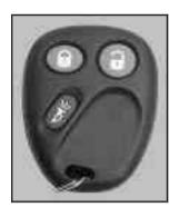
button on the remote keyless entry transmitter to lock the doors. This also arms the theft-deterrent system. See "Theft-Deterrent System" following for information on arming the theft-deterrent system.
