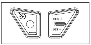
The buttons for the cruise control are located on the steering wheel.
