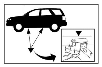
4. Position the lift head at the jack location nearest the flat tire. Make sure all of the jack lift head is touching the jacking flange under the body. Do not place the jack under a body panel. The lower body panel has an arrow to aid in locating the jacking location.
