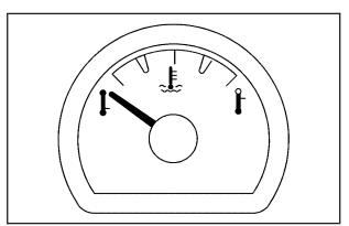
This gage measures the temperature of the vehicle's engine. If the indicator needle moves into the shaded area, the engine is too hot. A temperature indicator light will turn on.
