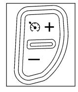
The buttons for the cruise control are located on the steering wheel.
