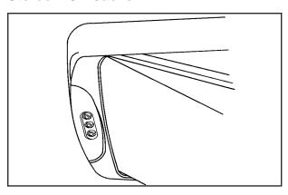
The RCA jacks are located behind the video screen on the overhead console. The RCA jacks allow audio or video signals to be connected from an auxiliary device such as a camcorder or a video game unit to the RSE. Adapter connectors or cables may be required to connect the auxiliary device to the RCA jacks. Refer to the manufacturer's instructions for proper usage.
