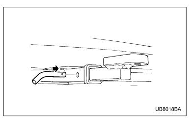
3. Insert the hitch pin into the hole on the hitch receiver tube so that the pin passes through the ball mount.
