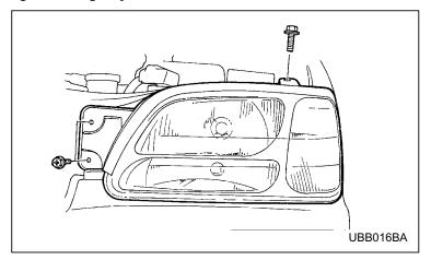
1. Remove the headlight assembly mounting screws located at the top of and the front of the headlight as-
