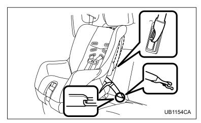
Some types of child restraint systems can be installed on the rear seat of your vehicle without use of the seat-belts. Such child restraint systems are secured to the dedicated anchorages provided on the vehicle body. The lower and tether anchorages are sometimes referred to as the LATCH system (Lower Anchors and Tethers for CHildren).
