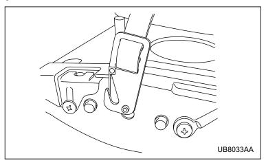
After you have rotated the bed extender, lock the black buckle pin into the tailgate latch by pushing downward until you hear two clicks. Then tighten the tether straps. Repeat this process for the other side. When you want to return the tailgate and the bed extender to the closed/inward position, pull on the tailgate release handle to disengage the tethers.
