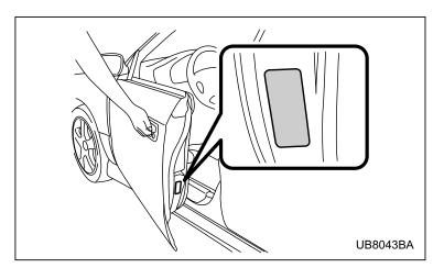
GVWR is shown on the certification label located on the driver's door of your vehicle.
