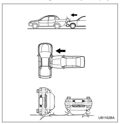
The SRS frontal airbag is basically not designed to deploy if the vehicle is struck from side or from behind, or if it rolls onto its side or roof, or if it is involved in a low-
