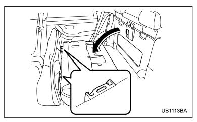
2. Unlock the rear seatback by pulling up on the knob and fold down the rear seatback. Confirm that the pins located at the bottom of the seat cushion is inserted into the slots at the top of the seatback.
