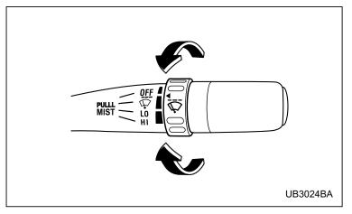
When the wiper switch is in the " \( \overline{\topi} \) " position, turn the dial to adjust the operating interval of the wiper. The operating interval can be adjusted continuously from the shortest interval to the longest.
