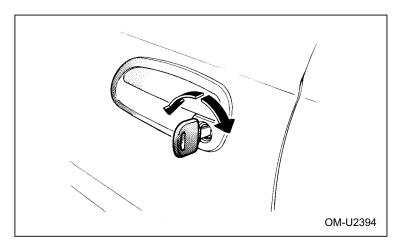
To lock the door from the outside with the key, insert the key into the keyhole and turn the key toward the rear. To unlock the door, turn the key toward the front.
