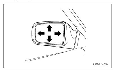
To adjust the mirrors by hand, push where indicated by the arrows.
