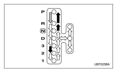
: When the brake pedal depressed, shift while pressing the button in.
