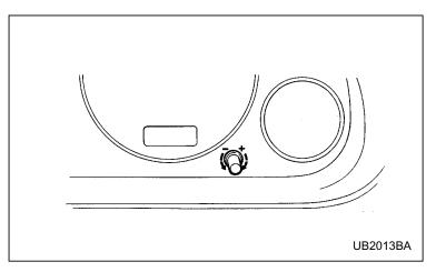
To set the time, turn the setting knob clockwise to advance and counterclockwise to retard the time.
