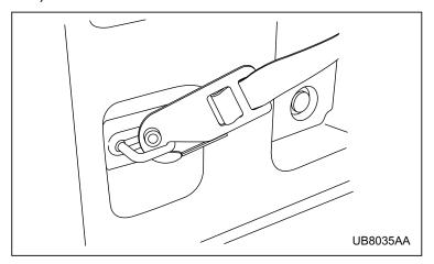
The bed extender should be secured to the rear set of vehicle cargo hooks. Latch the buckle onto the rear cargo hooks and then tighten the tether straps. To disengage the tethers, loosen the tether straps and de-
