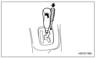
4. Insert the screwdriver into the hole.
