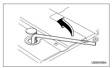
4. Turn the hoist shaft end counterclockwise with the wheel nut wrench until the temporary spare tire is on the ground with enough cable slack to allow you to pull it out from under the vehicle.
