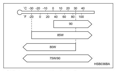
**SAE viscosity No. and Applicable Temperature**
