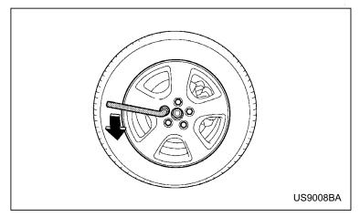
1. Loosen the wheel nuts using the wheel nut wrench
