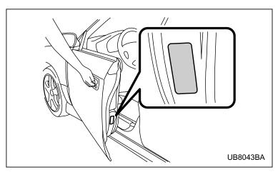
The certification label attached to the driver's side door shows GVWR (Gross Vehicle Weight Rating) and GAWR (Gross Axle Weight Rating).
