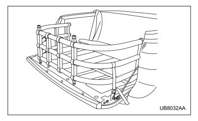
**Open/Outward Position** – To use the bed extender in the open/outward position, simply lower your license plate bracket (see section "License plate bracket" under heading of "Tailgate" in Chapter 2), open your tailgate, and rotate the bed extender until it sits on the tailgate.
