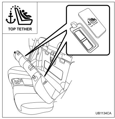
2. Pull the seatback locking knob and fold the seatback forward to see the tether anchorage on the backside of the seatback.
