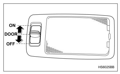
The dome light switch has three positions:
