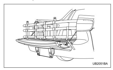
When you drive with the tailgate open and with the bed extender used, the license plate bracket must be placed at its fully lowered/open position to make the rear license plate visible.
