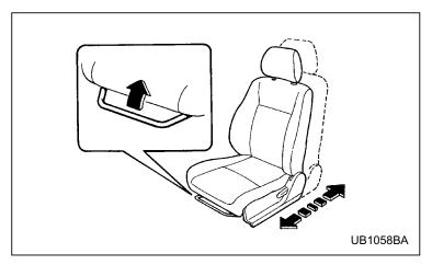
Pull the lever upward and slide the seat to the desired position. Then release the lever and move the seat-back and forth to make sure that it is securely locked into place.
