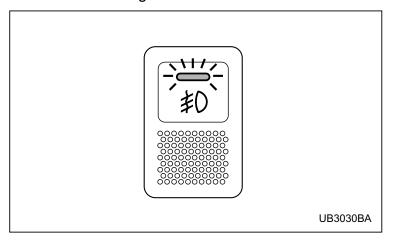
The indicator light located on the switch will illuminate when the fog lights are on.
