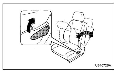
Pull the reclining lever up and adjust the seatback to the desired position. Then release the lever and make sure the seat is securely locked into place.
