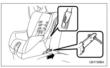
6. While following the instructions supplied by the child restraint system manufacturer, connect the lower hooks onto the lower anchorages located at " " marks on the bottom of the rear seatback. When the hooks are connected, make sure the adjacent seatbelts are not caught.
