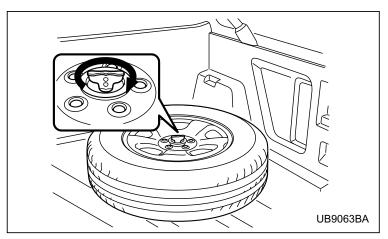
5. Secure the flat tire by tightening the tire holding rod.
