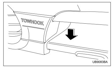
1. Free the tabs on the towing hook cover by firmly pressing the point indicated by an arrow with the palm of your hand.
