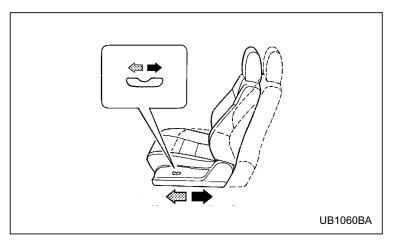
To adjust the seat forward or backward, move the control switch forward or backward.
