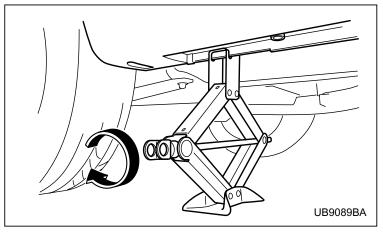
3. Turn the jackscrew by hand until the groove of the jack head engages firmly into the jack-up point.
