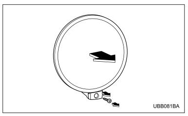
1. Remove front lamp screw and remove the lens and reflector.
