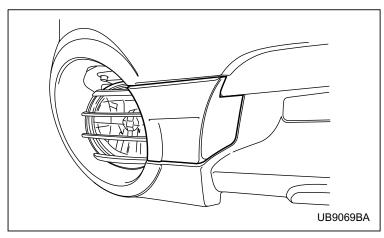
To reinstall the towing hook cover, push it in on both sides while pushing it back to its original position. Make certain that the tabs at the end of the cover are securely inserted into the corresponding slots in the vehicle's body.
