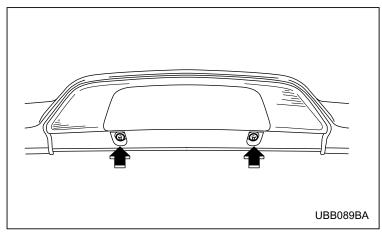
1. Remove the high mount stop light mounting screws.
