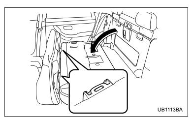
4. Unlock the seatback by pulling the release knob up and fold the seatback down. Confirm that the pin located at the bottom of the seat cushion is inserted into the slot at the top of the seatback.
