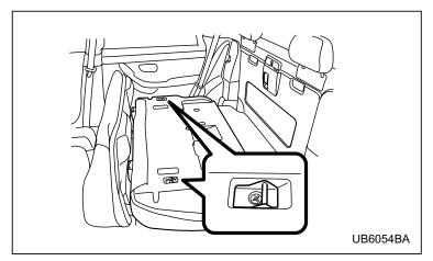
There are four hooks on the back panel behind the rear seatback.
