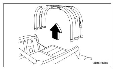
The bed extender can be removed from the vehicle by rotating the extender into a vertical position then lifting straight up.
