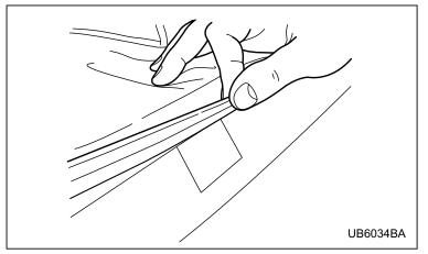
To secure the soft portion of the bed cover to the bed, simply start from either side of the vehicle and place the plastic strip under the rail. Slide your hand down the side of the vehicle pushing the plastic strip under the rail as you go. Continue this around the entire length of the bed. Fasten both closeout wraps with Velcro around the rear chrome bars so that they are secure. Your cover should be tight and ready to conceal items in the bed from view.
