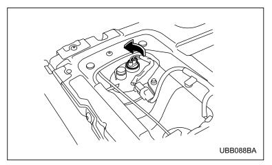
4. Remove the bulb socket from the tail light by turning it counterclockwise.
