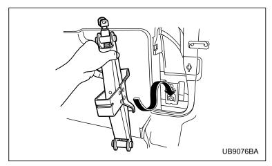
3. Place the jack onto the bracket in the pocket.
