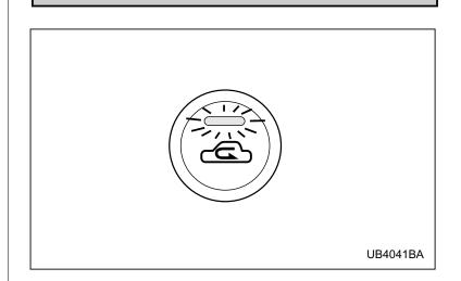
ON position (Recirculation): Interior air is recirculated inside the vehicle. Push the air inlet selection button to the ON position. The indicator light will come on. Push the air inlet selection button to the ON position for fast cooling with the air conditioner or when driving on a dusty road.
