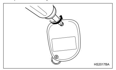
1. Remove the two screws on the back of the trans-
