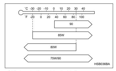
**SAE viscosity No. and Applicable Temperature**
