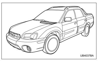
Always keep the front ventilator inlet grille free of snow, leaves, or other obstructions to ensure efficient heating and defrosting. Since the condenser is located in front of the radiator, this area should be kept clean because cooling performance is impaired by any accumulation of insects and leaves on the condenser.
