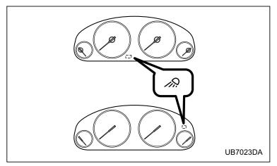
The cargo lamp comes on and goes off whenever the cargo lamp switch is pushed regardless of the position of the ignition switch. The cargo lamp indicator light located in the meter panel will illuminate when the cargo lamp is on.
