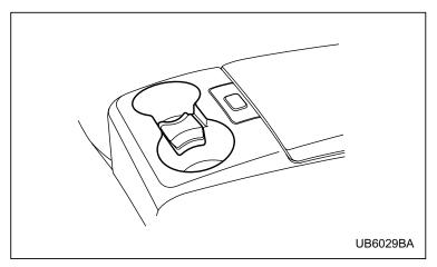
A dual cup holder is built in the rear center console.
