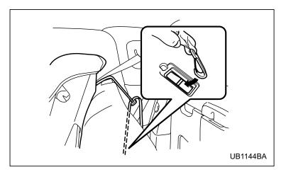
3. Connect the hook of the upper tether belt onto the tether anchorage on the backside of the seatback. Do not allow slack in the tether belt.
