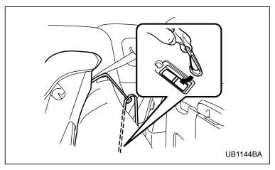
3. Connect the tether belt hook onto the tether anchorage on the backside of the seatback. Take up any slack in the tether belt after connecting it to the tether anchorage.
