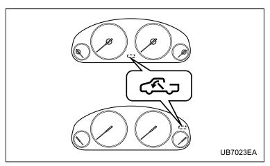
While the ignition switch is in the "ON" position, the switchback door indicator light comes on when the switchback door is open.
