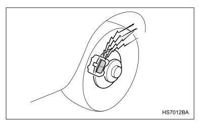
The front disc brakes and the right rear disc brake have an audible wear indicators on the brake pads. If the brake pads wear close to their service limit, the wear indicator makes a very audible scraping noise when the brake pedal is applied.
