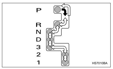
With the brake pedal depressed, move the lever along the gate.
