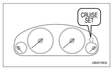
At this time, the "  $^{\text{CRUISE}}_{\text{SET}}$  " indicator light is illuminated in the combination meter.
