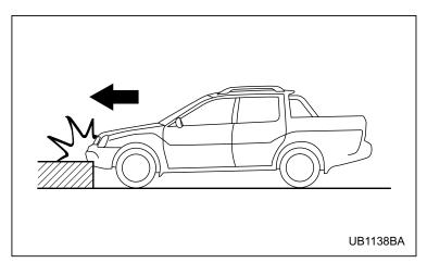
The SRS frontal airbag may be activated when the vehicle sustains a hard impact in the undercarriage area from the road surface (such as when the vehicle plunges into a deep ditch, is severely bumped or knocked hard against an obstacle on the road such as a curb).
