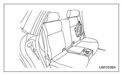
The jack and tool bag are located in the left side rear quarter pocket at the back side of the rear seatback.
