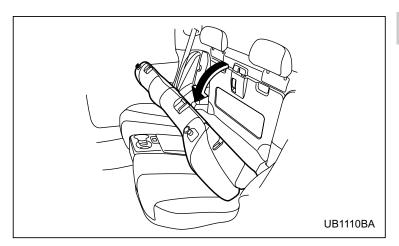
1. Unlock the seatback by pulling the release knob up and then fold the seatback down.
