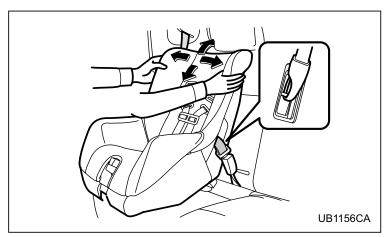
10. While pushing the child restraint into the seat cushion and moving it back and forth and right and left, tighten the seatbelt securely by taking up the slack in the belt.
