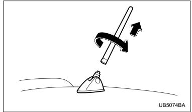
Stand the roof antenna up for use. You can detach the roof antenna by turning it counterclockwise. When fitting the roof antenna, turn it clockwise and tighten it securely.
