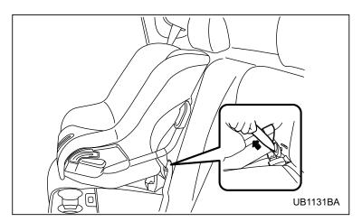
7. [If your child restraint system is of a flexible attachment type (which uses tether belts to connect the child restraint system properly to the lower anchorages)] While pushing the child restraint into the seat cushion, pull both left and right lower tether belts up to secure the child restraint system firmly by taking up the slack in the belt.
