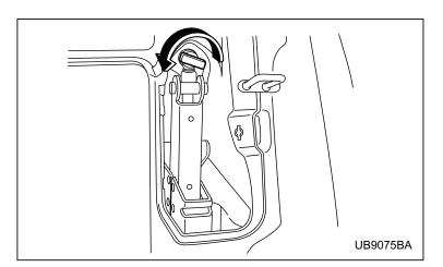
4. Loosen the jack holding screw by turning counterclockwise and remove the jack from the pocket.
