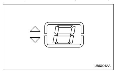
When the selector lever is in the manual gate, this indicator shows the currently selected gear.
