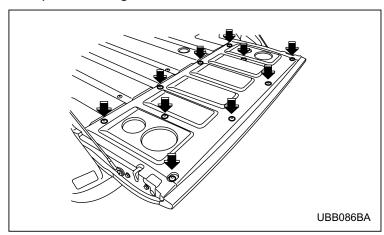
2. Remove the tailgate trim by loosening the installation screws.
