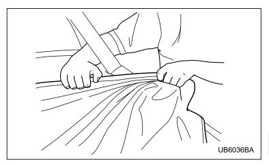
The soft portion of the bed cover can be removed from the bed cover's hard section for cleaning or storage. Unfasten the Velcro on the tube closeout wraps and firmly pull the cover out to one side.
