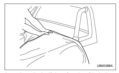
As you insert (and pull) the soft portion of the bed cover into the bed cover's hard section, make sure the next 10 to 15 inches (250 to 380 mm) of the soft portion are straight and ready to enter the flared out portion of the hard section.
