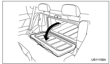
3. Fold down the switchback door by releasing the
