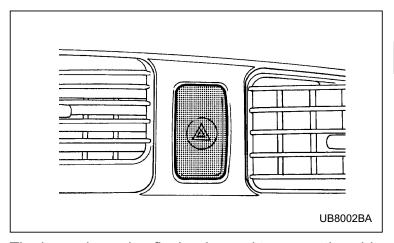
The hazard warning flasher is used to warn other drivers when you have to park your vehicle under emergency conditions. The hazard warning flasher works with the ignition switch in any position.
