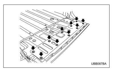
3. Remove the tail light cover by loosening the installation screws.
