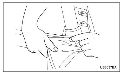
The soft portion of the bed cover can be reinstalled onto the bed cover's hard section. Start by inserting the left front edge of the soft portion into the right side of the hard cover. This area is flared out to ease installation.
