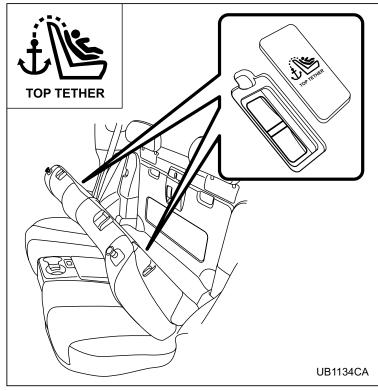
2. Unlock the rear seatback locking knob and fold the seatback forward to see the tether anchorages on the backside of the seatback.
