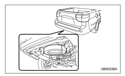
The spare tire is stored in the spare tire holder located under the rear of the cargo bed.
