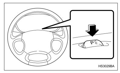
The parking light switch operates regardless of the ignition switch position.
