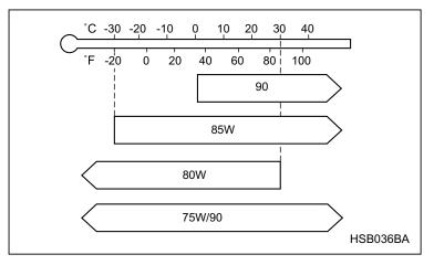
**SAE viscosity No. and Applicable Temperature**
