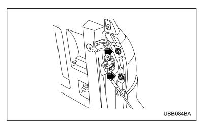
3. Remove the rear combination light mounting bolts. Then, slide the rear combination light assembly to the rear and remove it from the vehicle.
