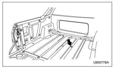
2. Remove the rubber cap from the cargo bed. Store the rubber cap in a safe place. Pay attention not to lose the rubber cap after removal.
