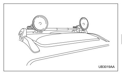
The sport activity lights mount to the vehicle front cross bar. The sport activity lights cross bar wire harness connects to the roof wire harness and then to the vehicle's electrical system.
