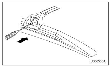
5. Adjust the alignment of the crossbar on the roof rails, and if available, use a T-30 torx® bit and torque wrench and tighten the T-30 torx® head screws to 30 to 35 lbf·in (3.4 to 4.0 N·m, 0.35 to 0.41 kgf·m) of torque (or tighten securely with the torx® wrench pro-
