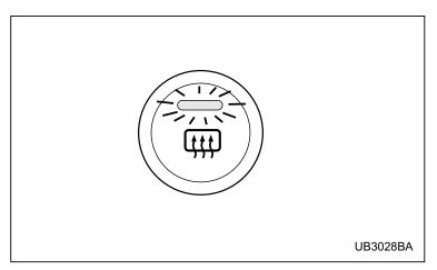
To turn on the defogger, push the switch. To turn it off, push the switch again.
