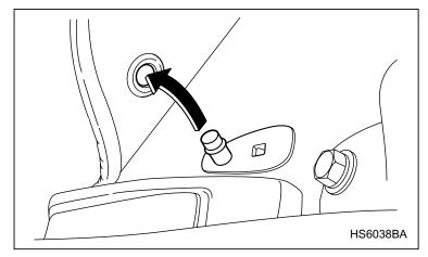
A retaining pin is located on the driver's side of the vehicle. The floor mat is secured using the built-in grommet, by placing the grommet over the pin and pushing downward.
