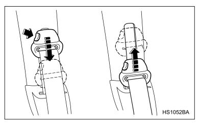
The shoulder belt anchor height should be adjusted to the position best suited for you. To lower the anchor height, push the release button and slide the anchor down. To raise the anchor height, slide the anchor up. Pull down on the anchor to make sure that it is locked in place.
