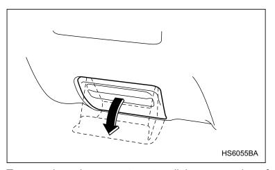
To open the coin compartment, pull the upper edge of the lid.
