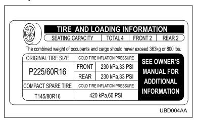
The vehicle placard shows original tire size, recommended cold tire inflation pressure on each tire at maximum loaded vehicle weight, seating capacity and loading information.
