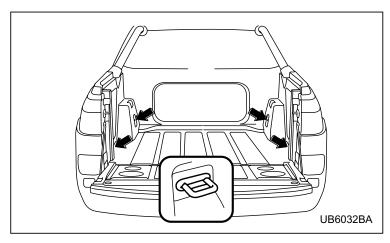
The cargo bed is equipped with four tie-down hooks so that cargo can be secured with a luggage net or ropes.
