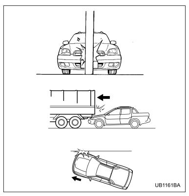
There are many types of collisions which might not necessarily require SRS frontal airbag deployment. If the vehicle strikes an object, such as a telephone pole
