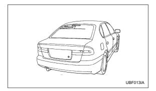
The antenna is printed on the inside of the rear window glass.
