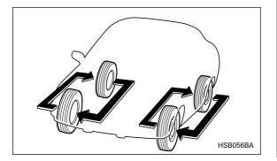
Tire wear varies from wheel to wheel. To maximize the life of each tire and ensure that the tires wear uniformly, it is best to rotate the tires every 7,500 miles (12,500 km). Rotating the tires involves switching the front and rear tires on the right-hand side of the vehicle and similarly switching the front and rear tires on the left-hand side of the vehicle. (Each tire must be kept on its original side of the vehicle.)
