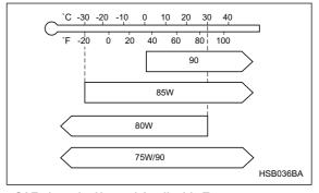
SAE viscosity No. and Applicable Temperature
