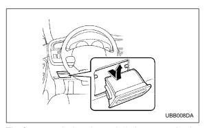
The fuses are designed to melt during an overload to prevent damage to the wiring harness and electrical equipment. The fuses are located in two fuse boxes. One is located under the instrument panel behind the coin tray on the driver's seat side.
