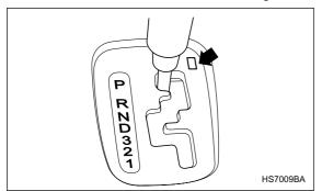
3. Remove the cover by prying on the edge with the regular screwdriver.
