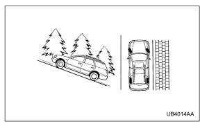
When parking on a hill, always turn the steering wheel. When the vehicle is headed up the hill, the front wheels should be turned away from the curb.
