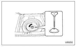
Turn the attaching bolt counterclockwise, then take spare tire out.
