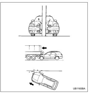
There are many types of collisions which might not necessarily require SRS frontal airbag deployment. If the vehicle strikes an object, such as a telephone pole or sign pole, or if it slides under a truck's load bed, or if it sustains an oblique offset frontal impact, the SRS frontal airbag may not deploy depending on the level of accident forces involved.
