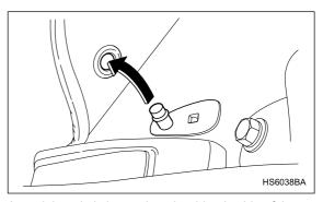
A retaining pin is located on the driver's side of the vehicle next to the fuel filler door release. The floor mat is secured using the built-in grommet, by placing the grommet over the pin and pushing downward.
