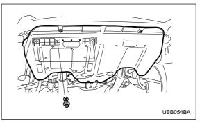
6. Remove three clips at the front of the cover under the oil filter.
