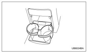
The rear passenger's cup holder is located on the lower side of the back of the center console. To use the cup holder, open the lid by pulling its upper edge.
