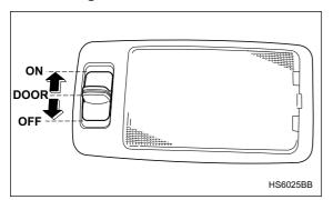
The dome light switch has three positions:
