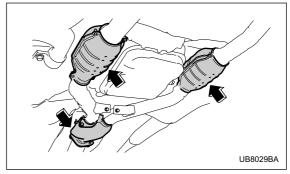
The catalytic converter is installed in the exhaust system. It serves as catalyst to reduce HC, CO and NOx in exhaust gases, thus providing cleaner exhaust.
