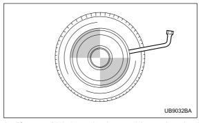
6. (If your vehicle has wheel covers) Insert the wheel nut wrench into the notch provided in the wheel cover, and pry it off.
