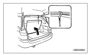
**Station wagon**: Open the lid and hang the hook provided on the underside of the lid on the rear edge of the roof to keep the lid open. Remove the storage tray.
