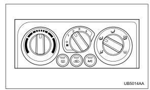
This setting allows you to direct air of different temperatures from the instrument panel and foot outlets. The air from the foot outlets is slightly warmer than from the instrument panel outlets.
