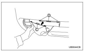
1. Insert the projection **C** into the hole **D**.
