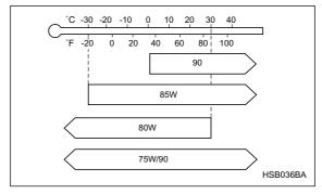
SAE viscosity No. and Applicable Temperature
