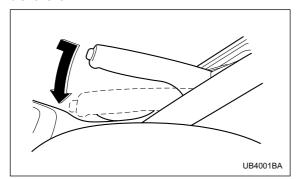
To release the parking brake, pull the lever up slightly, press the release button, then lower the lever while keeping the button pressed.
