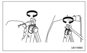
After placing the jack in its storage location, turn the jackscrew clockwise by hand until it becomes too hard to turn. Then, tighten it by an additional 1/4 – 1/3 of a turn using a screwdriver or the jack handle. Unless the jack is properly secured, it may rattle while the vehicle is moving.
