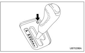
3. Remove the cover by prying on the edge with the regular screwdriver.
