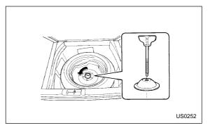
Turn the attaching bolt counterclockwise, then take the spare tire out.
