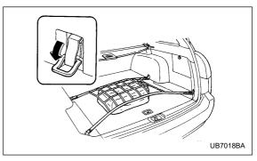
The cargo area is equipped with four tie-down hooks
