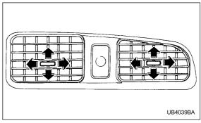
Move the thumb-wheel up and down or right and left to adjust the flow direction.
