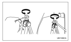
If the jackscrew is too tight to be loosened by hand, loosen it using a screwdriver or the jack handle. The jack handle is stored under the spare tire cover.
