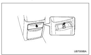
The rear ashtray is located on the upper side of the back of the center console. To open the ashtray, pull the upper edge of the lid.
