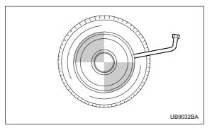
Insert the wheel nut wrench into the notch provided, and pry the wheel cover off.
