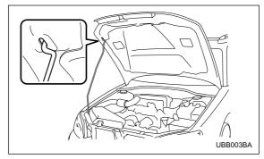
4. Lift up the hood, release the hood prop from its retainer and put the end of the hood prop into the slot in the hood.
