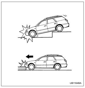
The SRS frontal airbag may be activated when the vehicle sustains a hard impact in the undercarriage area
