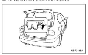
The inside trunk lid release can be cancelled to help prevent unauthorized entry into the trunk. To cancel the trunk lid release, set the lid release cancel lever (located on the inside of the trunk lid, mounted to the trunk lid latch) to the "CANCEL" position. When this lock is in the "CANCEL" position, the trunk can be opened only with the key.
