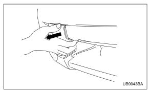
2. Press portion  ${\bf B}$  and simultaneously pull the towing hook cover toward you.
