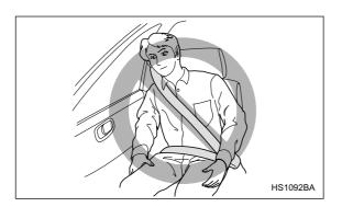
Do not sit or lean unnecessarily close to either front door. The SRS side airbag is stored in both front seat seatbacks next to the door, and it provides protection by deploying rapidly (faster than the blink of an eye) in the event of a side impact collision. However, the force of SRS side airbag deployment may cause injuries if your head or other body parts are too close to the SRS side airbag.
