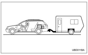
Vehicle capacity weight of the vehicle is 800 lbs (363 kg), which is indicated on the vehicle placard with the statement "The combined weight of occupants and cargo should never exceed 363 kg or 800 lbs".
