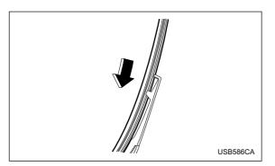
4. Align the claws of the plastic support with the grooves in the blade rubber assembly, then slide the blade rubber assembly into place.
