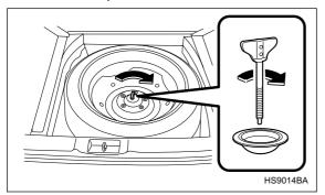
15. Store the flat tire in the spare tire compartment. When storing a conventional tire, put the spacer upside down and tighten the attaching bolt firmly. Also store the jack and wheel nut wrench in their storage locations.
