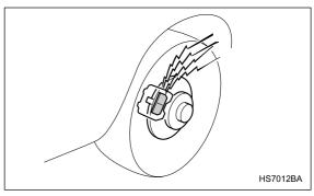
The disc brake pad wear warning indicators on the disc brakes give a warning noise when the brake pads are worn.
