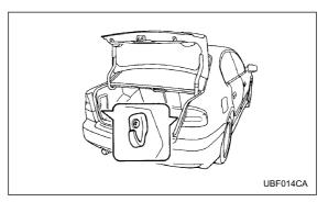
A shopping bag hook is attached to each inner side wall of the trunk near the trunk lid opening.
