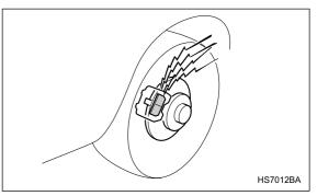
The front disc brakes and the right rear disc brake have an audible wear indicators on the brake pads. If the brake pads wear close to their service limit, the wear indicator makes a very audible scraping noise
