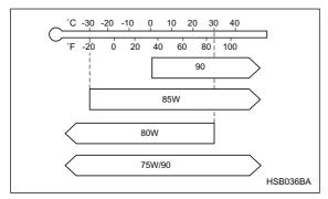
SAE viscosity No. and Applicable Temperature
