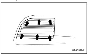
Align the towing hook cover with its original installation position and press all parts of it into place.
