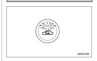
**ON position (Recirculation):** Interior air is recirculated inside the vehicle. Push the air inlet selection button to the ON position. The indicator light will come on. Push the air inlet selection button to the ON position for fast cooling with the air conditioner or when driving on a dusty road.
