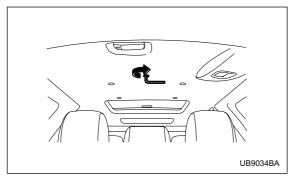
3. Insert the wrench in the end of the motor shaft. To close the moonroof, turn the wrench clockwise.
