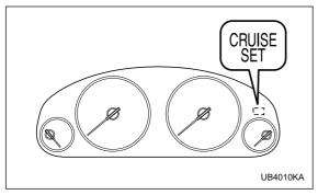
At this time, the " "" indicator light is illuminated in the combination meter.
