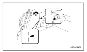
Electrical power (12V DC) from the battery is on tap at the outlet when the ignition switch is either in the "ACC" or "ON" position.
