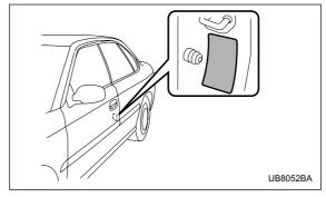
The load capacity of your vehicle is determined by weight, not by available cargo space. The maximum load you can carry in your vehicle is shown on the tire placard attached to the driver's side door jamb. It includes the total weight of driver and all passengers and their belongings, any optional equipment such as a trailer hitch, roof rack or bike carrier, etc., and the tongue load of a trailer.
