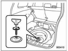
Turn the attaching bolt counterclockwise, then take the spare tire out.
