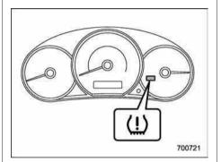
The tire pressure monitoring system provides the driver with a warning message by sending a signal from a sensor that is installed in each wheel when tire pressure is severely low.
