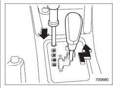
If you inadvertently have turned the ignition switch to the "LOCK" position with the selector lever in the "N" position, proceed as follows. To remove the shift lock release cover, refer to the "Shift lock release" section in this chapter. Then, with a screwdriver inserted into the hole, move the selector lever to the "P" position. If the selector lever reverse inhibiting function fails, have the vehicle inspected by the nearest SUBARU dealer.
