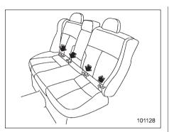
The lower anchorages (bars) are used for installing a child restraint system only on the rear seat window-side seating positions. For each window-side seating position, two lower anchorages are provided. Each lower anchorage is located where the seat cushion meets the seatback
