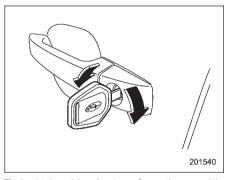
To lock the driver's door from the outside with the key, turn the key toward the rear. To unlock the door, turn the key toward the front.
