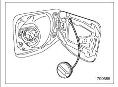
3. Hook the cord that is attached to the fuel filler cap onto the hook inside the fuel filler lid.
