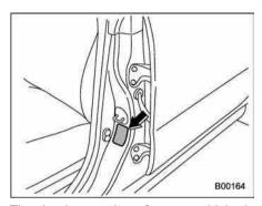
The load capacity of your vehicle is determined by weight, not by available cargo space. The maximum load you can carry in your vehicle is shown on the vehicle placard attached to the driver's side door pillar. It includes the total weight of the driver and all passengers and their belongings, any optional equipment such as a trailer hitch, roof rack or bike carrier, etc.
