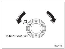
Turn the TUNE dial clockwise to increase the tuning frequency and turn the "TUNE" dial counterclockwise to decrease it.
