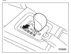
SPORT mode is used when power is needed for rapid acceleration or for uphill driving. To select this mode, move the selector lever from the "D" position to the manual gate.
