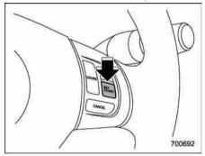
3. Push the "SFT/COAST" button and release it. Then release the accelerator pedal.
