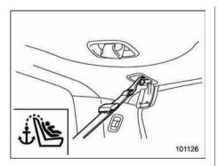
8. If the child restraint system requires a top tether, latch the hook onto the top tether anchorage and tighten the top tether. Refer to "Top tether anchorages" in this section for additional instructions.
