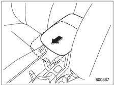
2. Push the armrest part of the console top forward to the desired position. Adjust the position of the armrest to suit your driving position. Make sure the armrest is securely retained.
