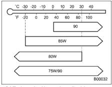
SAE viscosity No. and applicable temperature
