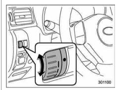
The brightness of clock display, audio, air conditioner, information display and instrument panel illumination dims when the light switch is in the "=co=" or "=co" or "=co" or "=co" or the instrument panel illumination for better visibility.
