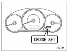
The cruise control set indicator light illuminates when the ignition switch is turned to the "ON" position and turns off after approximately 3 seconds.
