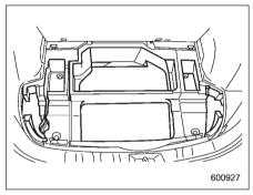
The storage compartment is located under the floor of the cargo area, and it can be used to store small items. To open the lid, pull the tab up.
