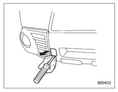
2. Pry off the cover on the front bumper using a screwdriver, and you will find a threaded hole for attaching the towing hook.
