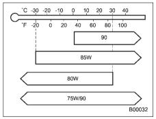
SAE viscosity No. and applicable temperature
