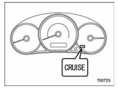
The cruise control indicator light illuminates when the ignition switch is turned to the "ON" position and turns off after approximately 3 seconds.
