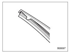
Securely retain both ends of the rubber with the stoppers on the plastic support ends. If the rubber is not retained properly, the wiper may scratch the rear window class.
