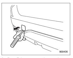
2. Prv off the cover on the rear bumper using a screwdriver, and you will find a threaded hole for attaching the towing hook.
