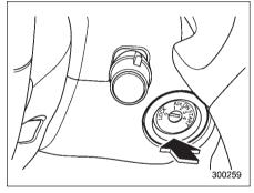
The ignition switch has four positions: LOCK, Acc. ON and START.
