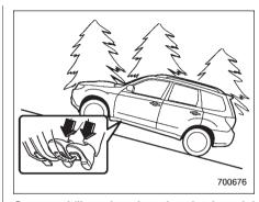
On an uphill grade, when the clutch pedal is depressed while the brake pedal is also depressed, braking power is maintained temporarily by the Hill start assist system when the brake pedal is released. The driver is therefore able to start the vehicle the same way as on a level grade, just using the clutch and accelerator pedal.
