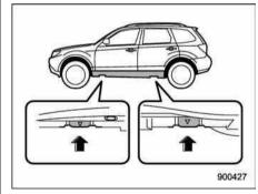
7. Place the jack under the side sill at the front or rear jack-up point closest to the flat tire.
