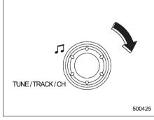
Turn the "TRACK" dial clockwise to skip to the beginning of the next track/file (track). Each time the dial is turned, the indicated track/file (track) number will increase.
