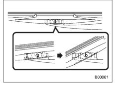
2. Turn the wiper blade assembly counterclockwise.
