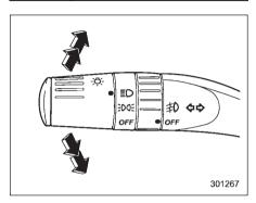
To activate the right turn signal, push the turn signal lever up. To activate the left turn signal, push the turn signal lever down. When the turn is finished, the lever will return automatically. If the lever does not return after cornering, return the lever to the neutral position by hand.
