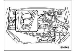
Check the fluid level on the outside of the reservoir. If the level is below "MIN" level mark, add the recommended clutch fluid to "MAX" level mark.
