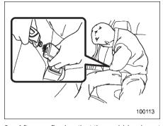
3. After confirming that the webbing is not twisted, insert the connector (tongue) attached at the webbing end into the buckle on the right-hand side until a click is heard.
