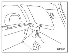
1. Remove the cover of the retainers by prying on the edge with a flat-head screwdriver.
