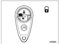
Press the "a" button to lock all doors and the rear gate. An electronic chirp will sound once and the turn signal lights will flash once.
