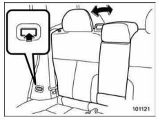
Push the switch and adjust the seatback to the desired position.
