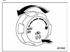
**ON position (Recirculation):** Interior air is recirculated inside the vehicle. Push the air inlet selection button to the ON position for fast cooling with the air conditioner or
