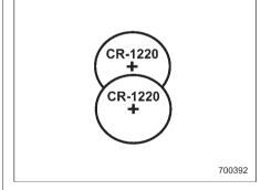
2. Remove the circuit board from the bottom half of the case and slide the white plastic battery holder out from under the battery tab releasing the batteries. Remove the old batteries and replace with new ones. Be sure to observe the (+) sign
