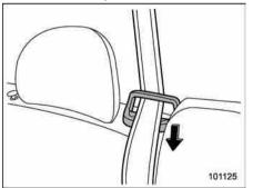
2. After drawing out the seatbelt, pass it through the belt guide.
