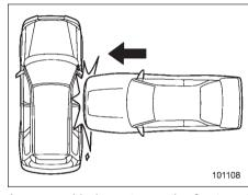
A severe side impact near the front seat activates the SRS side airbag and SRS curtain airbag.
