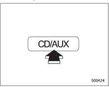
Press the "AUX" button when the auxiliary audio input is off to turn on the auxiliary audio input.
