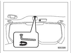
2. Insert a hex-head wrench in the end of the motor shaft.
