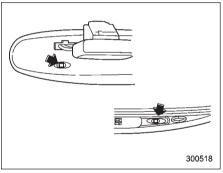
The mirror has a photosensor attached on both the front and back sides. If the glare from the headlights of vehicles behind you strikes the mirror, these sensors detect it and make the reflection surface of the mirror dimmer to help prevent you from being blinded. For this reason, use care not to cover the sensors with stickers, or other similar items. Periodically wipe the
