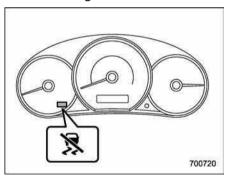
This single light has the function of indicating malfunctions in the Vehicle Dynamics Control system and the function of indicating that the Vehicle Dynamics
