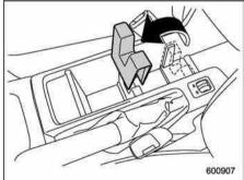
The cup holder rear partition can be removed and placed on the front partition. This space can be used to store small items.
