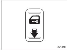
6. When you have finished entering the number, push the unlock side of the lock switch within 5 seconds.
