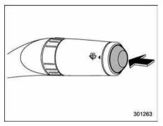
To wash the windshield, push the washer button at the end of the wiper control lever. The washer fluid sprays until you release the washer button. The wipers operate while you push the button.
