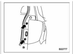
7. Tighten the upper and lower screws.
