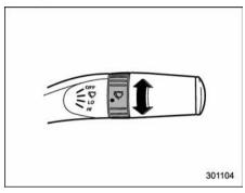
When the wiper switch is in the "T" position, turn the dial to adjust the operating interval of the wiper.
