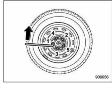
13. Use the wheel nut wrench to securely tighten the wheel nuts to the specified torque, following the tightening order in the illustration.
