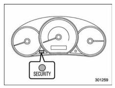
The security indicator light deters potential thieves by indicating that the vehicle is equipped with an immobilizer system. It begins flashing (approximately once every 3 seconds) approximately 60 seconds after the ignition switch is turned from the "ON" position to the "Acc" or "LOCK" position or immediately after the key is pulled out.
