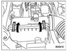
3. Unsnap the two clips holding the air cleaner case cover.
