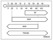
SAE viscosity No. and applicable temperature
