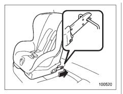
2. While following the instructions supplied by the child restraint system manufacturer, connect the lower hooks onto the lower anchorages located at "Q" marks on the bottom of the rear seatback. When the hooks are connected, make sure the adjacent seatbelts are not caught.
