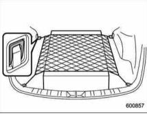
The cargo area is equipped with four tiedown hooks so that cargo can be secured with a cargo net or ropes.
