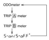
\*: "5-an" or "5-aFF" cannot be displayed when the ignition switch is in the "ON" position.
