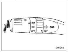
To change from low beam to high beam, push the turn signal lever forward. When the headlights are on high beam, the high beam indicator light "\( \bar{\su} \) on the combination meter is also on.
