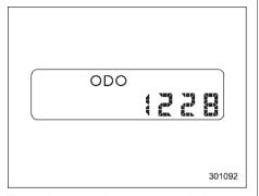
The odometer shows the total distance that the vehicle has been driven.
