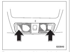
To turn on the map light, push the lens. To turn it off, push the lens again.
