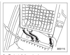
6. To install the air cleaner case cover, insert the three projections on the air cleaner case cover into the slits on the air cleaner case and then snap the two clips on the air cleaner case cover.
