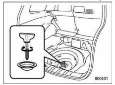
14. Store the flat tire in the spare tire compartment. Put in the spacer and tighten the attaching bolt firmly.
