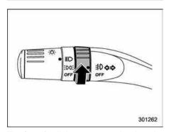
The front fog lights operate only when the low beam headlights are illuminated. However, the front fog lights turn off when the headlights are switched to high beam. To turn on the front fog lights, turn the front fog light switch on the turn signal lever upward to the "红" position. To turn off the front fog lights, turn the switch back down to the "OFF" position.
