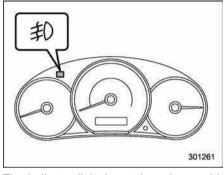
The indicator light located on the combination meter will illuminate when the front fog lights are on.
