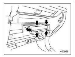
3. Replace the air filter element with a new one.
