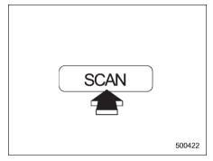
Press the "SCAN" button to change the radio to the SCAN mode. In this mode, under the selected category, the radio scans through the channel until a station is found. The radio will stop at the station for 5 seconds while displaying the channel number, after which scanning will continue until the entire channel has been scanned from the low end to the high end.
