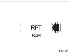
To playback a track/file(s) at random, press the "RPT" button for 0.5 second or longer while the track/file is playing. Each time you press the button, the mode changes in the following sequences.
