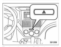
The hazard warning flasher is used to warn other drivers when you have to park your vehicle under emergency conditions. The hazard warning flasher works regardless of the position of the ignition switch.
