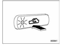
**ON position (Recirculation):** Interior air is recirculated inside the vehicle. Push the air inlet selection button to the ON position. The indicator light will illuminate.
