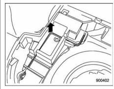
The jack handle is stored under the floor cover of the cargo area.
