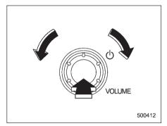
The dial is used for both power (ON/OFF) and volume control. The radio is turned ON and OFF by pushing the dial, and the volume is controlled by turning the dial.
