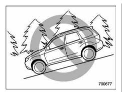
The Hill start assist system does not operate when the vehicle is facing down-hill. And the Hill start assist system may not operate on slight grades.
