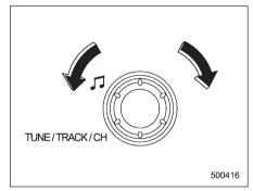
Turn the "CH" dial clockwise to select the next channel and turn the "CH" dial counterclockwise to select the previous channel.
