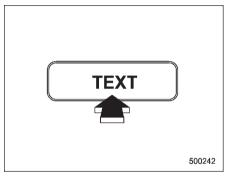
If the PS (Program Service Name) and/or RT (Radio Text) are available, pressing the "TEXT" button changes the display among PS, RT and frequency. The initial setting is "PS".
