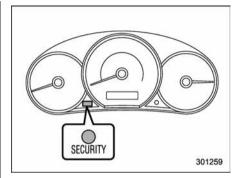
6. Briefly press the "P" button (for less than 2 seconds). All doors and the rear gate will lock, an electronic chirp will sound once, the turn signal lights will flash once, and the indicator lights will start flashing rapidly. After rapid flashing for 30 seconds (standby time), the indicator lights will then flash slowly (twice approximately every 2 seconds), indicating that the system has been armed for surveillance.
