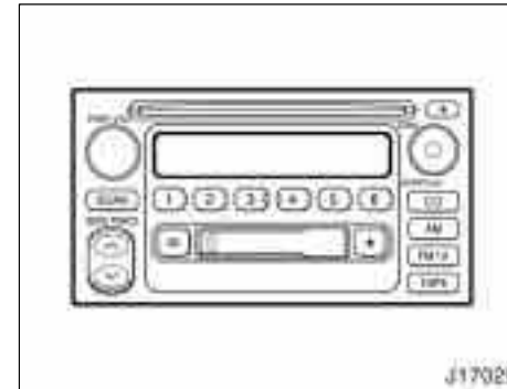
Type 2-2: AM-FM ETR radio/cassette player/compact disc player (with compact disc auto changer controller)
