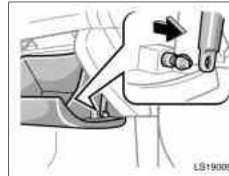
1. Open the glove box, and slide off the damper as shown.
