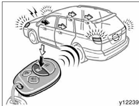
Unlocking operation (type A)
