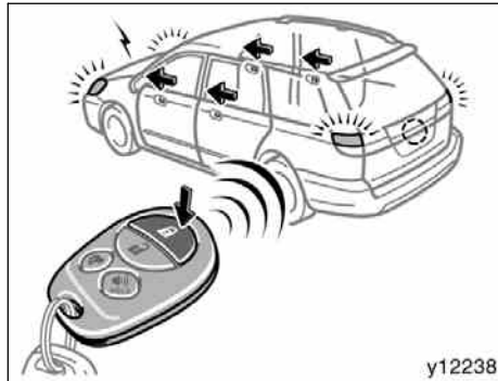
Locking operation (type A)
