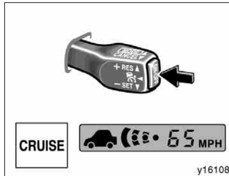
Vehicle-to-vehicle distance control mode
