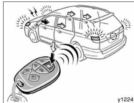
Unlocking operation (type B)
