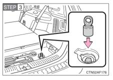
Attach the adapter socket (for removing a spare tire) on the spare tire clamp bolt.
