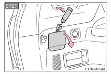
Open the back door and remove the cover.
