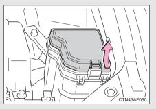
Type A: Push the tab in and lift the fuse box cover off.
