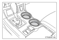
Removing the adapters changes the size. ( $\rightarrow$ P. 381)
