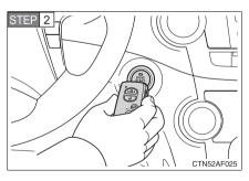
Touch the Toyota emblem side of the electronic the kev to "ENGINE START STOP" switch.
