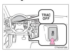
Quickly push and release the button to turn off TRAC.
