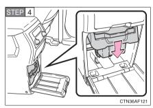
Push down on the end to engage the pins in the holes and close the console box door.
