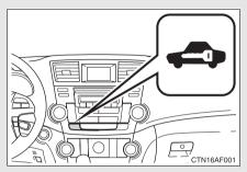
Close the doors and hood, and lock all doors using the wireless remote control door lock function or entry function (vehicles with smart key system). The system will be set automatically after 30 seconds.
