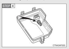
Remove the fuse with the pullout tool.
