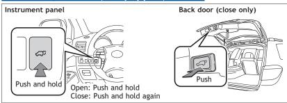
**NOTE:** If battery is disconnected, the power back door needs to be reinitialized. Refer to the *Owner's Manual* for more details.
