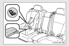
Second seat: Child restraint LATCH anchors
