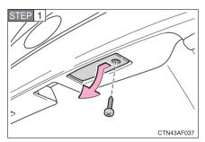
Remove the screw and remove the unit.
