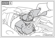
Add engine coolant if necessary.
