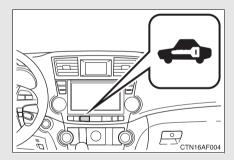
Close the doors and hood, and lock all doors using the wireless remote control door lock function or entry function (vehicles with smart key system). The system will be set automatically after 30 seconds.
