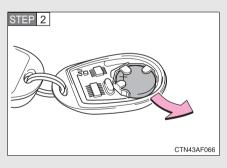
Remove the discharged transmitter battery.
