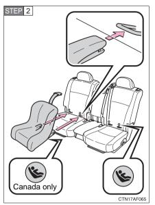
Latch the buckles onto the LATCH anchors.
