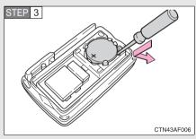
Remove the depleted battery.
