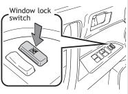
**Automatic operation (driver's window only)** Push the switch completely down or pull it completely up and release to fully open or close. To stop window midway, lightly push the switch in the opposite direction.
