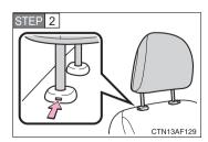
Push a flathead screwdriver into the slot. (The slot is located on the opposite side of the head restraint to the lock released button.)
