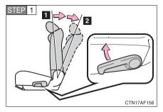
Fold the seatback while pulling the lever. Return the seatback and secure it at the 1st lock position (most upright position). Adjust the seatback to the 3rd lock position.  $(\rightarrow P.~82)$
