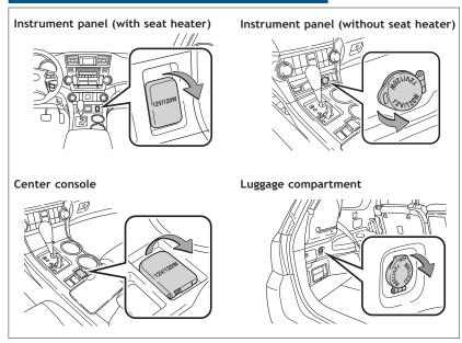
Key/Engine switch must be in the "ACC" or "ON" position to be used.
