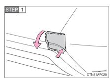
Remove the eyelet cover while pushing it.
