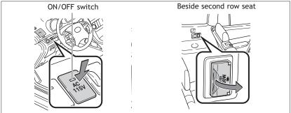
Key/Engine switch must be in the "ON" position to be used.
