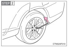
Slightly loosen the wheel nuts (one turn).
