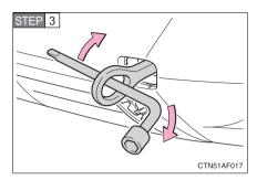
Tighten down the towing eyelet using a wheel nut securely wrench.
