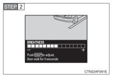
Press the "DISP" button to adjust the brightness.
