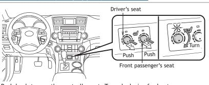
Push knob to pop the controller out. Turn clockwise for heater.
