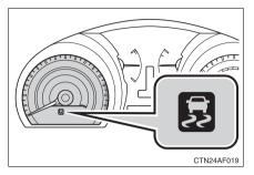
If the vehicle is in danger of slipping, rolling backwards when starting on an incline, or the front wheels (2WD models) or four wheels (4WD models) spin, the indicator flashes to indicate that the Enhanced VSC/TRAC systems have been engaged.
