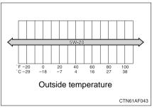
Recommended oil viscosity (3.5 L V6 (2GR-FE) engine)
