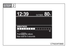
Press the "DISP" button to adjust the brightness.
