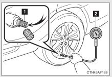
STEP 1 Remove the tire valve cap.
