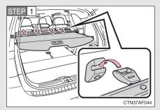
Hang the hooks on the hook brackets on the second seat seatback.
