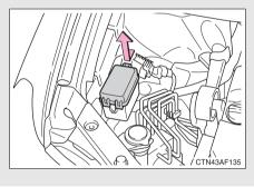
Type B: Push the tab in and lift the fuse box cover off. (if equipped)
