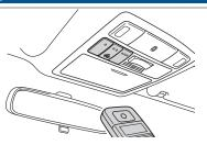
Garage door openers manufactured under license from HomeLink®\* can be programmed to operate garage doors, estate gates, security lighting, etc.
