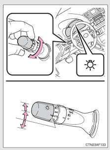
The side marker, parking, tail, license plate and instrument panel lights turn on.
