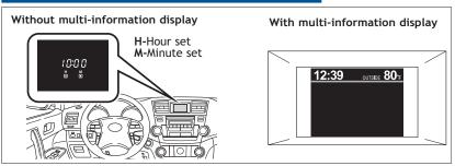
With multi-information display Press and hold "DISP" button. Select "CLOCK" on menu screen. Adjust as indicated on screen.
