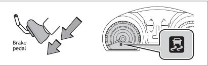
HAC helps prevent rolling backwards on an incline. To engage, push further down on brake pedal while at a complete stop until a beep sounds and slip indicator illuminates. HAC holds for approximately 2 seconds after releasing brake pedal.
