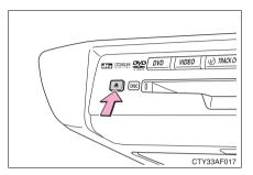
Press (a) and remove the disc.
