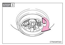
Release the bulb retaining spring.
