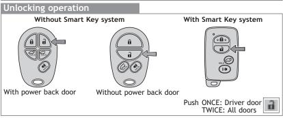
**NOTE:** If a door is not opened within 60 seconds of unlocking, all doors will relock for safety.
