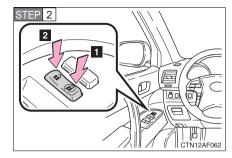
Shift the shift lever to P or N, and press and hold the driver's door lock switch (1 or 2) for approximately 5 seconds and then release it.
