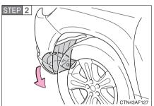
Remove the fender liner.
