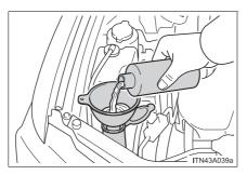
If any washer does not work or the low washer fluid warning light comes on, the washer tank may be empty. Add washer fluid.
