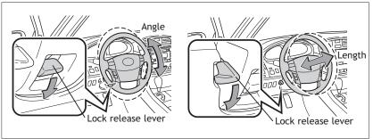
Hold wheel, push lever down, set angle and length, and return lever.
