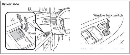
**Automatic operation** Push the switch completely down or pull it completely up and release to fully open or close. To stop window midway, lightly push the switch in the opposite direction.
