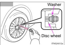
Install the spare tire and loosely tighten each wheel nut by hand to approximately the same amount.
