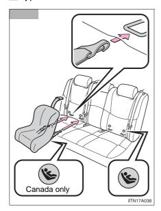
Latch the hooks of the lower straps onto the LATCH anchors.
