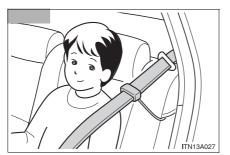
Buckle, position and release the seat belt.
