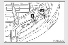
Adjustment bolt AAdjustment bolt B
