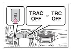
Quickly push and release the button to turn off TRAC/TRC.
