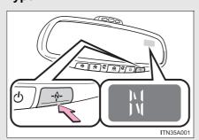
To turn the compass on or off, press the switch.
