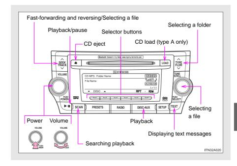
Loading and ejecting MP3 and WMA discs
