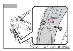
Remove the fender liner clip.
