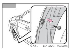
Remove the fender liner clip.
