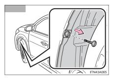
Remove the fender liner clip.
