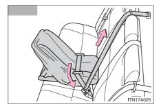
While pushing the child restraint system down into the rear seat, allow the shoulder belt to retract until the child seat is securely in place.
