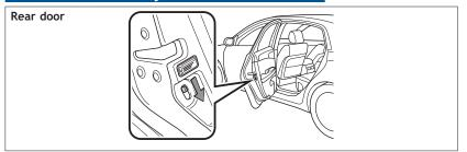
Moving the lever to "LOCK" will allow the door to be opened only from the outside.
