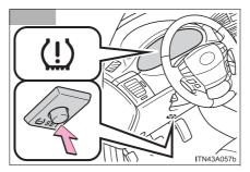
Push and hold the tire pressure warning reset switch until the tire pressure warning light blinks slowly 3 times.
