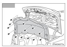
Open the trunk and remove the trunk panel cover.
