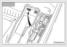
Remove the fuse with the pullout tool.
