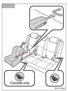
Latch the buckles onto the LATCH anchors.
