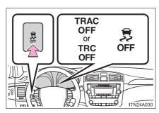
Push and hold the button for more than 3 seconds while the vehicle is stopped to turn off TRAC/TRC and VSC.
