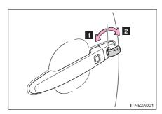
Using the mechanical key (→P. 24) in order to perform the following operations:
