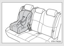
Seat belts equipped with a child restraint locking mechanism (ALR/ELR belts except driver's seat belt) (→P. 68)
