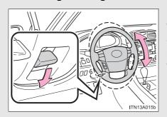
Hold the steering wheel, press the tilt lock release lever, and adjust to the ideal position by moving the steering wheel vertically.
