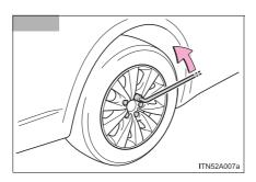
Slightly loosen the wheel nuts (one turn).
