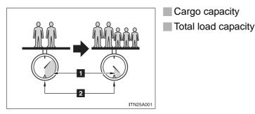
When 2 people with the combined weight of 366 lb. (166 kg) are riding in your vehicle, which has a total load capacity of 870 lb. (395 kg), the available amount of cargo and luggage load capacity will be as follows:
