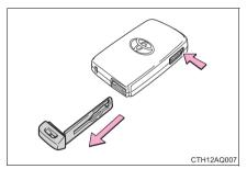
After using the mechanical key, store it in the electronic key. Carry the mechanical key together with the electronic key. If the electronic key battery is depleted or the entry function does not operate properly, you will need the mechanical key.  $(\rightarrow P. 476)$
