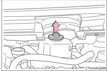
Add brake fluid slowly while checking the fluid level.
