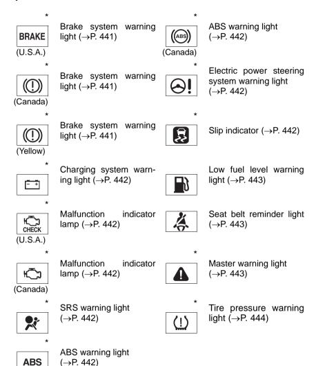
\*: These lights turn on when the engine switch is turned to the "ON" position (vehicles without a smart key system) or the "POWER" switch is turned to ON mode (vehicles with a smart key system) to indicate that a system check is being performed. They will turn off after the hybrid system is on, or after a few seconds. There may be a malfunction in a system if the lights do not come on, or turn off. Have the vehicle inspected by your Toyota dealer.
