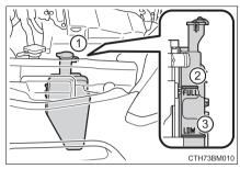
Power control unit coolant reservoir
