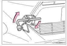
6 Securely attach a cable or chain to the towing eyelet. Take care not to damage the vehicle body.
