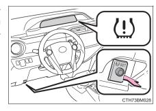
5 Vehicles without a smart key system: Wait for a few minutes with the engine switch in the "ON" position and then turn the engine switch to the "ACC" or "LOCK" position.
