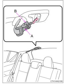
With tab "B" inserted all the way into the cover, move tab "A" slightly back toward the cover's inlet, so that it blocks the inlet.
