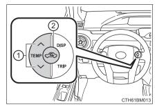
The mode switches between outside air mode and recirculated air mode each time (a) is pressed.
