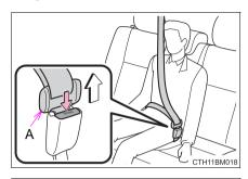
2 To release tab "B", insert the key (→P. 118) or tab "A" into the hole on the buckle.
