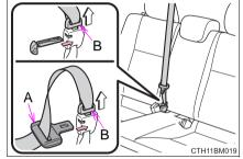
3 Holding tab "A" and "B" together, insert both tabs all the way into the cover on the roof.
