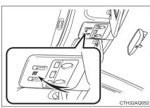
The vehicle's built in microphone is used when talking on the phone.
