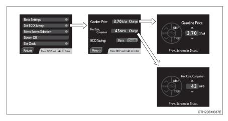
The gasoline price and fuel consumption comparison settings can be set, and the screen settings can be changed between basic and detailed.
