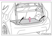
2 Remove the spare wheel cushions, then loosen the center fastener that secures the spare tire.
