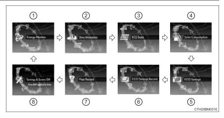
Each time the "DISP" switch is pressed, the menu screen changes. When the desired menu screen is displayed, stop pressing the "DISP" switch. The details screen will soon be displayed.
