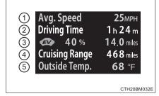
EV driving rate and driven distance (percentage and distance driven using just the electric motor [traction motor] only) will be displayed.
