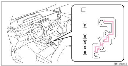
Vehicles without a smart key system: While the engine switch is in the "ON" position, move the shift lever with the brake pedal depressed.
