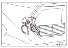
5 Tighten down the towing eyelet securely using a wheel nut wrench.
