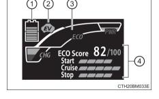
Driving conditions are displayed in 5 stages and divided into 3 categories: start, cruise and stop. Every time the vehicle is stopped, the score is displayed. (Every time the vehicle is accelerated the score that was last displayed is reset. Accumulative scores are not calculated.)
