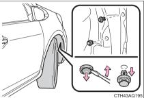
3 Partly remove the fender liner.
