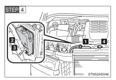
The coolant level is satisfactory if it is between the "FULL" and "LOW" lines on the reservoir.
