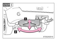
Confirm that the tire is not loose after tightening:
