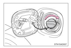
After refueling, turn the fuel tank cap until you hear a click. Once the cap is released, it will turn slightly in the opposite direction.
