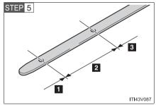
Holding a rag under the end, pull the dipstick out and check the oil level.
