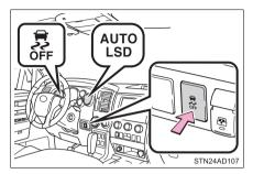
Stop the vehicle completely, and press the VSC OFF switch for more than 3 seconds, when the system is in the TRAC OFF mode.
