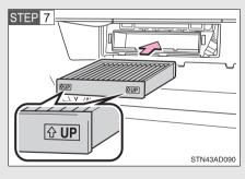
Remove the air conditioning filter and replace it with a new one.
