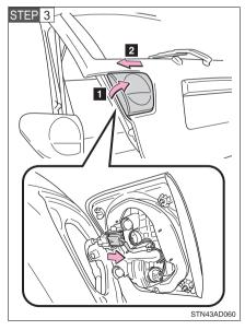
Remove the rear combination light assembly in the order shown in the illustration.
