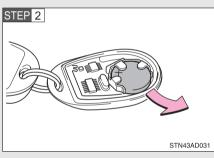
Remove the discharged transmitter battery.
