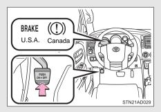
the parking Set brake\*. (Depressing the pedal again releases the parking brake.)
