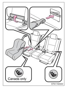
Latch the hooks of the lower straps onto the LATCH anchors and tighten the lower straps.
