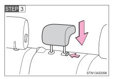
Adjust the center head restraint to the downmost position.
