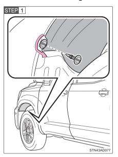
Remove the fender liner clip.
