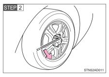
Slightly loosen the wheel nuts (one turn).
