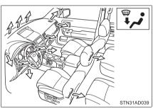
When the dial is set to , air flows to the feet and the wind-shield defogger operates.
