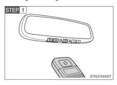
Point the remote control transmitter for the device 1 to 3 in. (25 to 75 mm) from the HomeLink<sup>®</sup> control buttons.
