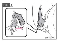
Remove the bolts and partly remove the fender liner.
