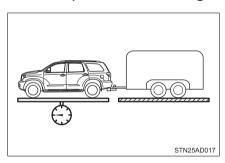
The maximum allowable gross vehicle weight. The gross vehicle weight is the total weight of the vehicle. When towing a trailer, it is the sum of the vehicle weight (including the occupants, cargo and any optional equipment installed on the vehicle) and the tongue weight.
