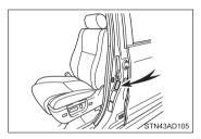
For the GAWR, see the Certification Label. For the maximum load of the tire, see the load limit at maximum cold tire inflation pressure mentioned on the sidewall of the tire.  $(\rightarrow P. 528)$
