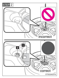
Lay down the tire with the valve stem facing up and install the holding bracket, inserting the claw into the wheel lug nut hole. Turn the jack handle extension clockwise to take up slack in the chain.
