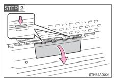
Remove the cover and loosen the strap.
