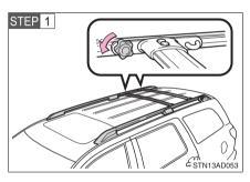
Turn the knobs counterclockwise to loosen the cross rails.
