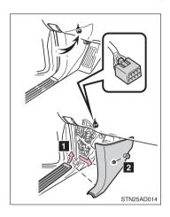
Your vehicle is equipped with a service connector for the trailer brake controller as shown.
