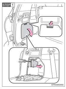
Open the back door and remove the covers.
