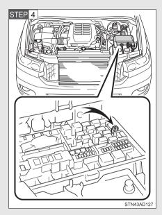
Remove the fuse with the pullout tool.
