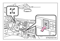
Use the center differential lock system if your wheels get stuck in a ditch, or when you are driving on a slippery or bumpy surface.
