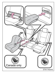
Fold the seatback while pulling the lever. Return the seatback and secure it at the 1st lock position (most upright position). Adjust the seatback to the 8th lock position. (→P. 51)
