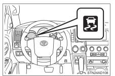
If the rear wheels spin, the slip indicator flashes to indicate that the AUTO LSD system has controlled the spinning of the rear wheels
