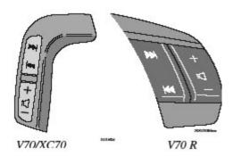
4. Press the AUTO button or the arrow keys on the optional steering wheel controls briefly to select the stored stations. When the radio is in auto-store mode, AUTO is shown in the display. AUTO disappears when you return to the normal radio mode.
