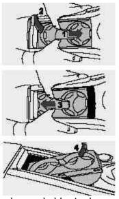
Removing the cup holder in the center console
