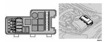
A - To open, press the plastic catches on the sides of the fuse box cover and lift
