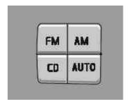
This function automatically searches for and stores up to 10 strong AM or FM stations in a separate memory. If more than ten stations are found, the ten strongest ones are stored. This function is especially useful in areas in which you are not familiar with radio stations or their frequencies.
