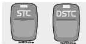
Press this switch to turn the Spin Control (SC) function of the STC/DSTC system on or off. To help reduce the risk that the SC function is turned off inadvertently, the switch must be held in for at least half a second to disable this function.
