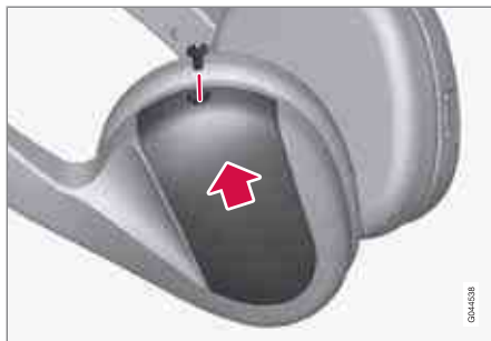
Battery cover and retaining screw
