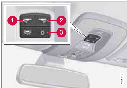
Light switches, front roof lighting
