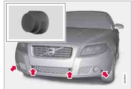
Location of the front sensors
