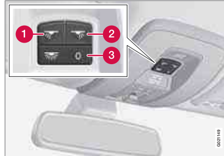
Light switches, front roof lighting
