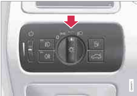
Light switch in the AUTO position
