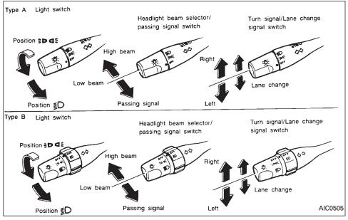
To select the high beam function, push the lever forward. The high beam lights come on and the indicator light illuminates. Pull it back to select the low beam.
