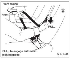
Pull on the shoulder belt until all of the belt is fully extended. At this time, the seat belt retractor is in the automatic locking mode (child restraint mode). It reverts back to emergency locking mode when the seat belt is fully retracted.
