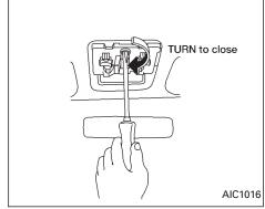
3. Using a wide blade screwdriver, turn the shaft clockwise to close the sunroof.
