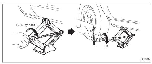
2. Place the jack directly under the jack-up point as illustrated above so the top of the jack contacts the vehicle at the jack-up point. Align the jack head between the two notches in the front or the rear as shown. Also fit the groove of the jack head between the notches as shown.
