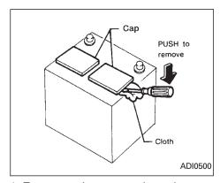
To remove the cap, gently pry between the battery cap and cover as illustrated.
