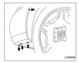
Remove the four screws from the bottom of the front fender protector (see above illustration) and position the fender protector aside to allow access to the headlamp mounting fasteners.
