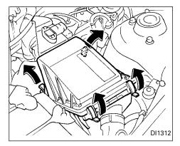
The air cleaner filter should not be cleaned and reused. Replace it according to the maintenance intervals shown in the "Maintenance" section of this manual. When replacing the filter, wipe the inside of the air cleaner filter housing and the cover with a damp cloth.
