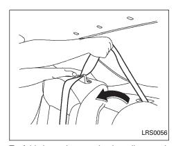
To fold down the seat back, pull approximately 10 inches of seat belt webbing out of the retractor and hold, then unlatch and fold down the seat back.
