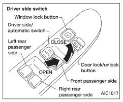
The power windows operate only when the ignition key is in the ON position. To open a window, press down on the switch. To close a window, pull up on the switch. To stop the opening or closing function at any time, simply release the switch.
