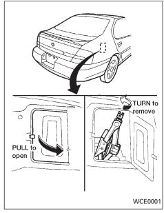
2. Push the release clip on the jack access door to open. To remove the jack, turn the jack screw counterclockwise. Use either end of the jack rod to loosen the jack from its storage position.
