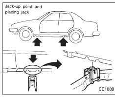
Jacking up vehicle and removing the damaged tire
