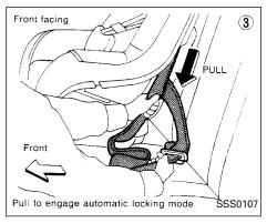
Pull on the shoulder belt until all of the belt is fully extended. At this time, the seat belt retractor is in the automatic locking mode (child restraint mode). It reverts back to emergency locking mode when the seat belt is fully retracted.
