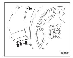
Remove the four screws from the bottom of the front fender protector (see above illustration) and position the fender protector aside to allow access to the headlamp mounting fasteners.
