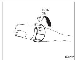
To turn the front fog lights on, rotate the switch to the  $\not\equiv \bigcirc$  position.
