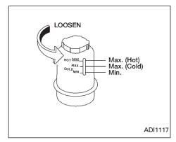
The fluid level should be checked using the HOT MAX range on the power steering fluid reservoir at fluid temperatures of 122° to 176°F (50° to 80°C) or using the COLD MAX range on the power steering fluid reservoir at fluid temperatures of 32° to 86°F (0 to 30°C).
