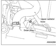
Check the radiator drain plug and the drain plug on the engine water pipe for any sign of leakage, tighten if necessary.
