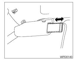
Slide the sun visor extension in or out as needed (if so equipped).
