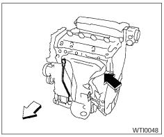
**QR25DE** engine **ENGINE SERIAL NUMBER**
