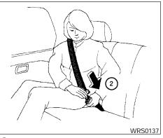
Slowly pull the seat belt out of the retractor and insert the tongue into the buckle until you hear and feel the latch engage.
