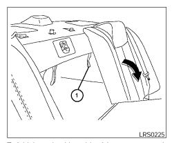
To fold down the driver side of the rear seat, reach through the opening and pull on the strap (1) located behind the seat.
