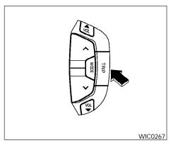
When the ignition switch is turned to ON, modes of the trip computer can be selected by pushing the trip mode switch on the steering wheel switch for audio controls or by the trip computer change button. The following modes can be selected:
