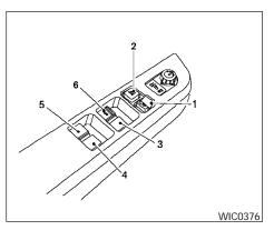
is opened during this period of about 45 seconds, power to the windows is canceled. To open a window, push the switch and hold it down. To close a window, pull the switch up. To stop the opening or closing function at any time, simply release the switch.
