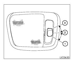
The interior light has a three-position switch and operates regardless of ignition switch position.
