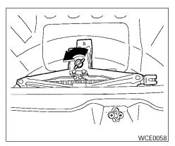
6. Unscrew the jack hold down and remove the jack.
