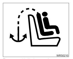
Flaps are provided in the carpet for easy access to the anchor point locations and are marked with the label shown.
