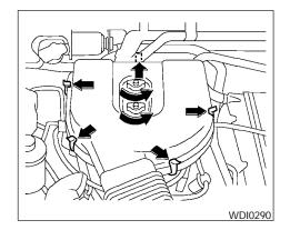
The air cleaner filter should not be cleaned and reused. Replace it according to the maintenance log shown in the "NISSAN Service and Maintenance Guide." When replacing the filter, wipe the inside of the air cleaner filter housing and the cover with a damp cloth.
