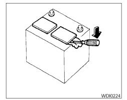
1. Remove the battery caps with a screwdriver as shown. Use a cloth to protect the battery case.
