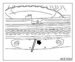
7. Find the oval-shaped opening above the middle of the license plate. Pass the T-shaped end of the jack rod through the opening and direct it toward the spare tire winch, located directly above the spare tire.
