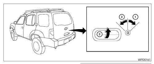
To unlock the back door, turn the key clockwise ①. To open the back door, lift up on the door handle ② and lift the door up. To close, lower and push the door down securely. To lock the back door, turn the key counterclockwise ③.
