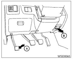
**To engage:** Firmly depress the parking brake (A)
