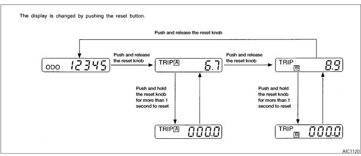
The trip odometer records the distance of individual trips. Before each trip reset the trip odometer.
