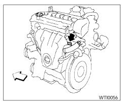
**KA24DE** engine **ENGINE SERIAL NUMBER**
