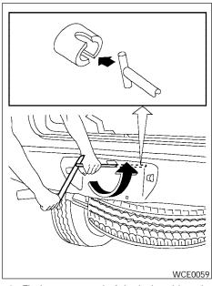
8. Fit the square end of the jack rod into the square hole of the wheel nut wrench to form a handle.
