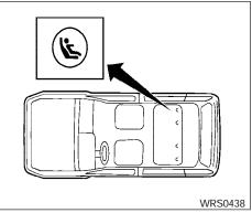
**LATCH** system anchor point locations LATCH (Lower Anchors and Tethers for CHildren) SYSTEM
