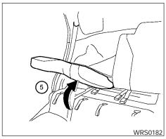
To return the rear seatback to a seating position, push the seatback up until it latches.
