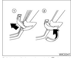
Pull the handle forward to unlock (1), then push the handle up completely to lock the sunroof closed (2).
