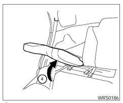
To return the rear seat to the normal position, push the seatback up until latches.
