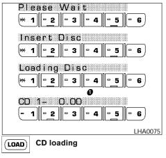
Press the LOAD button to start CD loading mode.
