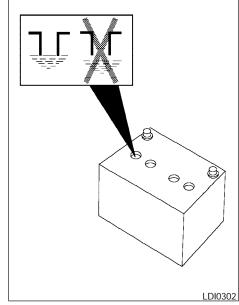
2. Check the fluid level in each cell If it is necessary to add fluid, add only distilled water to bring the level up to the bottom of the filler opening. Do not overfill.
