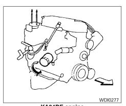
**KA24DE** engine CHANGING ENGINE OIL FILTER
