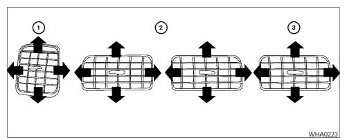
Adjust air flow direction for the driver side (1), center (2), and passenger side (3) ventilators by moving the ventilator slide and/or ventilator assemblies.
