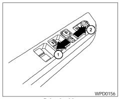
Driver's side LOCKING WITH POWER DOOR LOCK SWITCH (if so equipped)
