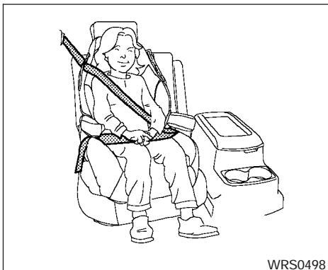
Booster seat installation on 2nd row captain's chairs (if so equipped)
