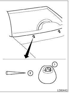
If you wax the surface of the hood, be careful not to let wax get into the washer nozzle (1). This may cause clogging or improper windshield washer operation. If wax gets into the nozzle, remove it with a needle or small pin (2).
