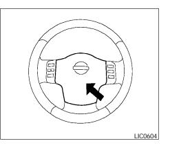
To sound the horn, push the center pad area of the steering wheel.
