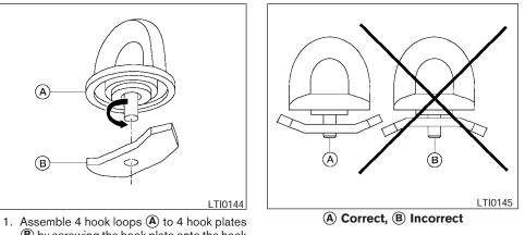
Assemble 4 hook loops (A) to 4 hook plates (B) by screwing the hook plate onto the hook (5 revolutions).
