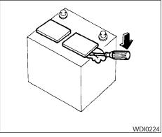
1. Remove the battery caps with a screwdriver as shown. Use a cloth to protect the battery case.
