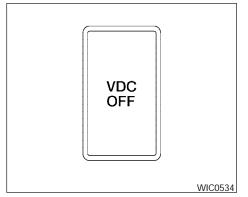
The vehicle should be driven with the Vehicle Dynamic Control (VDC) system on for most driving conditions.
