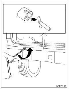
4. Fit the square end of the jack rod into the square hole of the wheel nut wrench to form a handle.
