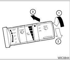
The rear window wiper and washer operate when the ignition switch is in the ON position.
