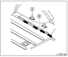
Insert (at any position) 2 channel tie-down hooks (A) into the channel opening (B) of each channel and slide to the desired position.
