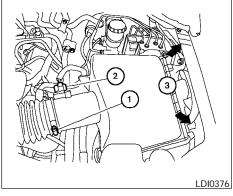
The air cleaner filter should not be cleaned and reused. Replace it according to the maintenance log shown in the "NISSAN Service and Maintenance Guide." When replacing the filter, wipe the inside of the air cleaner filter housing and the cover with a damp cloth.
