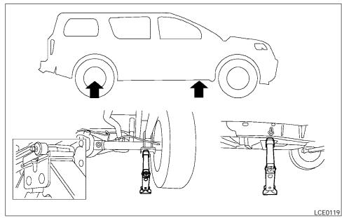
2. Place the jack directly under the jack-up point as illustrated so the top of the jack contacts the vehicle at the jack-up point. The front tire jack-up points are indicated by stamped arrows on the side of the frame. The jack should be used on firm and level ground.
