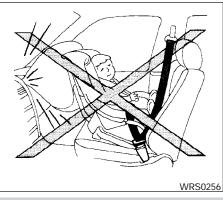
• Even with the NISSAN Advanced Air Bag System, never install a rear-facing child restraint in the front seat. An inflating supplemental front air bag could seriously injure or kill your child. See "Child restraints" earlier in this section for details.
