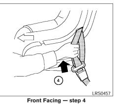
(4) Allow the seat belt to retract. Pull up on the shoulder belt to remove any slack in the belt.
