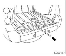
3. Find the oval-shaped opening above the middle of the bumper. Pass the T-shaped end of the jack rod through the opening and direct it toward the spare tire winch, located directly above the spare tire.
