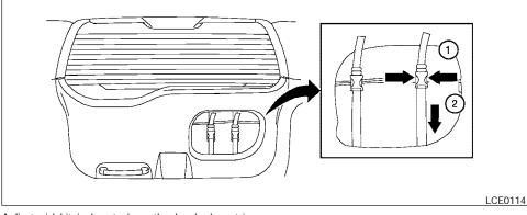
A first aid kit is located on the back door trim panel. To remove the first aid kit:
