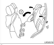
(2) Then pull the straps located on the outside edge of each seatback to fold the seatbacks forward.
