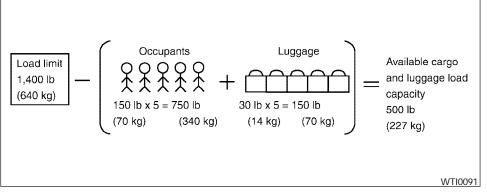
Steps for determining correct load limit
