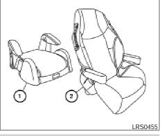
• Do not use towels, books, pillows or other items in place of a booster seat. Items such as these may move during normal driving or a collision and result in serious injury or death. Booster seats are designed to be used with a lap/shoulder belt. Booster seats are designed to properly route the lap and shoulder portions of the seat belt over the strongest portions of a child's body to provide the maximum protection during a collision.
