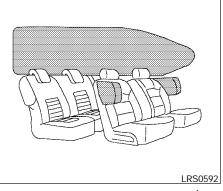
curtain side-impact and rollover air bags are designed to inflate in higher severity side collisions, although they may inflate if the forces in another type of collision are similar to those of a higher severity side impact. They are designed to inflate on the side where the vehicle is impacted. They may not inflate in certain side collisions.
