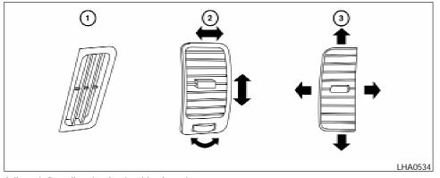
Adjust air flow direction for the driver's and passenger's side windows (1), driver and passenger (2), or center (3) ventilators by moving the ventilator slide and/or ventilator assemblies.
