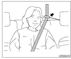
2. Insert the shoulder belt into the back of the comfort guide so that the seat belt lays flat in the guide. Be sure that the comfort guide routes the seat belt properly over the center of your shoulder and across your chest. The belt should be away from your face and neck, but not falling off of your shoulder.
