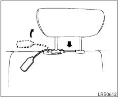
3. To return the seat belt comfort guide to the stowed position, route the comfort guide strap in the channel under the 2nd row driver's side seating position head restraint and attach the guide in the clip.
