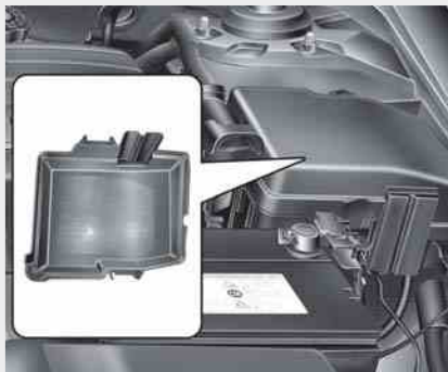
Engine compartment fuse panel
