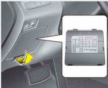
Inner panel fuse panel
