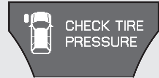
This shows that front left tire is losing pressure.
