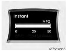
Instant fuel consumption (MPG or *l*/100km) This mode calculates the instant fuel consumption every 2 seconds (supervision type: every 0.2 second) from the driving distance and quantity of fuel injection.
