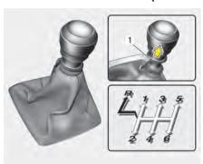
The shift lever can be moved into any of the forward gears without pulling the ring (1).
