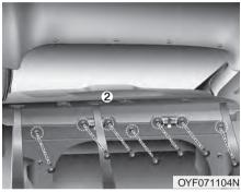
10. After loosening the mounting screws, then remove the package tray trim (2).
