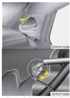
8. Take the C-pillar out carefully. If you pull the C-pillar strongly, it will be broken.
