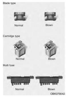
A vehicle's electrical system is protected from electrical overload damage by fuses. This vehicle has 2 fuse panels, one located in the driver's side panel bolster, the other in the engine compartment.
