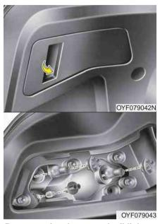
Rear turn signal, stop and tail light, side marker
