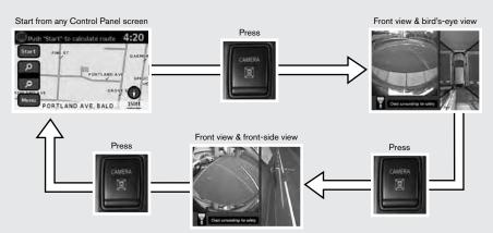
■ When the shift lever is in the **R** (**REVERSE**) position and the **CAMERA** button of is pressed, the following views will display in order:
