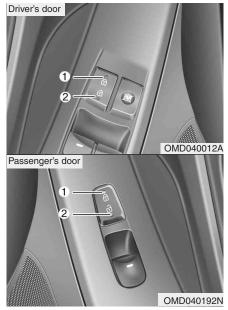
With central door lock switch (if equipped)
