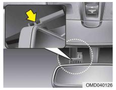
Auto defogging system (if equipped) Auto defogging reduces the probability of fogging up the inside of the windshield by automatically sensing the moisture of inside the windshield.
