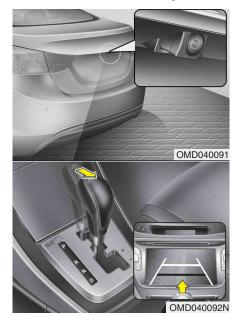
The rearview camera will activate when the back-up light is ON with the ignition switch ON and the shift lever in the R position.
