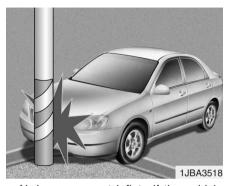
Air bags may not inflate if the vehicle collides with objects such as utility poles or trees, where the point of impact is concentrated to one area and the full force of the impact is not delivered to the sensors.
