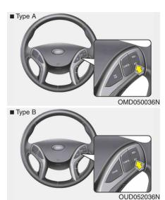
Push the SET- switch, and release it at the desired speed. The SET indicator light in the instrument cluster will illuminate. Release the accelerator at the same time. The desired speed will automatically be maintained.
