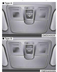
If your vehicle is equipped with a sunroof, you can slide or tilt your sunroof with the sunroof control switch located on the overhead console.
