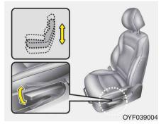
Seat cushion height (for driver's seat) To change the height of the seat cushion, push the lever upwards or downwards.
