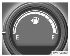
WARNING - Fuel gauge Running out of fuel can expose vehicle occupants to danger. You must stop and obtain additional fuel as soon as possible after the warning light comes on or when the gauge indicator comes close to the E level.
