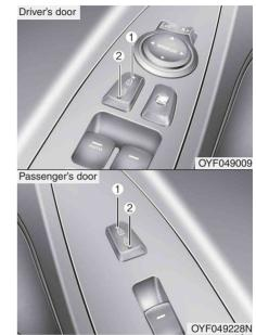
With central door lock switch Operate by depressing the central door lock switch.
