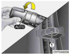
Auto light position (if equipped) When the light switch is in the AUTO light position, the taillights and headlights will be turned ON or OFF automatically depending on the amount of light outside the vehicle.
