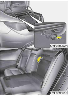
5. Pull on the seatback folding lever located in the trunk, then fold the seat toward the front of the vehicle. 6. To use the rear seat, lift and pull the seatback rearward. Push the seatback firmly until it clicks into place. Make sure the seatback is locked in place.
