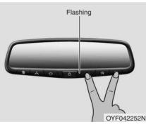
1. For first-time programming, press and hold the two outside buttons ((,,),), HomeLink<sup>®</sup> Channel 1 and Channel 3, until the indicator light begins to flash (after 10 seconds). Release both buttons. Do not hold the buttons for longer than 20 seconds.
