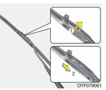
2. Lift up the wiper blade clip. Then pull down the blade assembly and remove it.
