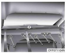
10. After loosening the mounting screws, then remove the package tray trim (2).
