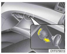
2. With the glove box open, remove the stoppers by turning them counter-clockwise on both sides.
