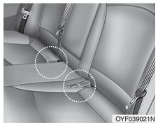
Stowing the rear seat belt The rear seat belt buckles can be stowed in the pocket between the rear seatback and cushion when not in use.
