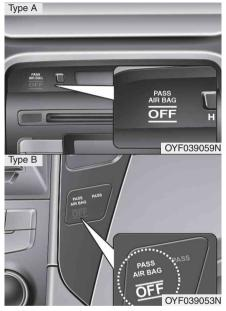
The occupant classification system is designed to detect the presence of a properly-seated front passenger and determine if the passenger's front air bag should be enabled (may inflate) or not. The driver's front air bag is not affected or controlled by the occupant classification system.
