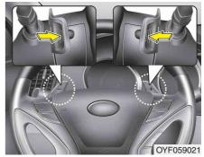
**Paddle shifter (if equipped)** The paddle shifter is available when the shift lever is in the D position or the sport mode.
