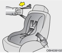
3. Pull the shoulder portion of the seat belt all the way out. When the shoulder portion of the seat belt is fully extended, it will shift the retractor to the "Aautomatic locking" (child restraint) mode.
