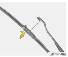
3. Install the new blade assembly in the reverse order of removal.
