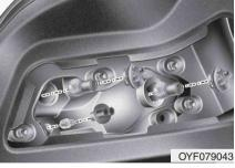
Rear turn signal, stop and tail light, side marker
