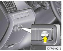
To open the trunk from inside the vehicle, press the trunk lid release button.
