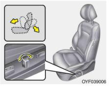
Seat cushion height (for driver's seat) Pull the front portion of the control switch up to raise or push down to lower the front part of the seat cushion. Pull the rear portion of the control switch up to raise or push down to lower the rear part of the seat cushion. Release the switch once the seat reaches the desired position.
