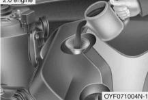
If it is near or at L, add enough oil to bring the level to F. **Do not overfill.**
