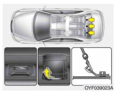
Securing a child restraint seat with "Tether Anchor" system Child restraint hook holders are located on the package tray.
