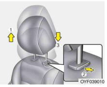
Adjusting the height up and down To raise the headrest, pull it up to the desired position (1). To lower the headrest, push and hold the release button (2) on the headrest support and lower the headrest to the desired position (3).
