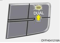
Adjusting the driver and passenger side temperature individually
