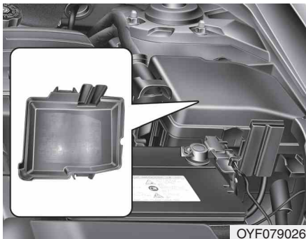
Engine compartment fuse panel (2.0 TGD)
