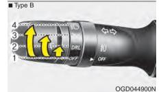
To operate the lights, turn the knob at the end of the control lever to one of the following positions:
