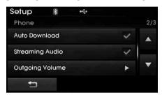
This feature is used to automatically download mobile contacts entries once a *Bluetooth®* Wireless Technology phone is connected.
