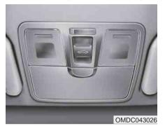
The ignition switch must be in the ON position before you can open or close the suproof
