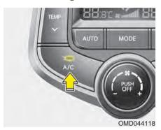
Push the A/C button to turn the air conditioning system on (indicator light will illuminate).
