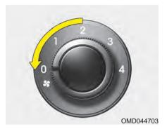
To turn off the fan, turn the fan speed control knob to the "0" position.
