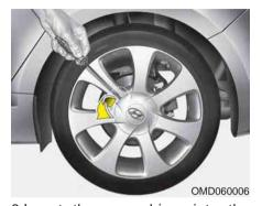
6.Insert the screwdriver into the groove of the wheel cap and pry gently to remove the wheel cap (If equipped).
