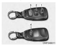
Your HYUNDAI uses a remote key, which you can use to lock or unlock a door (and trunk).
