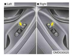
While the engine is running, push either switch to warm the rear seat. During mild weather or under conditions where the operation of the seat warmer is not needed, keep the switches in the "OFF" position.
