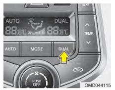
Adjusting the driver and passenger side temperature individually
