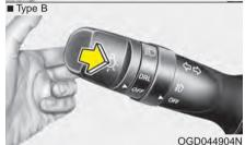
To flash the high beam headlights, pull the lever towards you, then release the lever. The high beams will remain ON as long as you hold the lever towards you.
