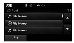
Turn the **TUNE** knob left/right to search for files. Once the desired file is displayed, press the knob to select and play.
