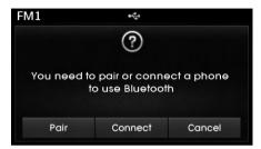
If Bluetooth® Wireless Technology devices are paired but none are currently connected, pressing the PHONE key or the key or the steering wheel displays the following screen. Press the [Pair] button to pair a new device or press the [Connect] to connect a previously paired device.
