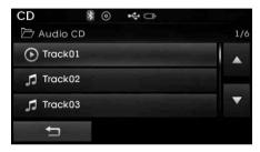
Turn the **TUNE** knob left/right to search for tracks. Once the desired track is displayed, press the knob to select and play.
