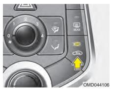
This is used to select outside (fresh) air position or recirculated air position
