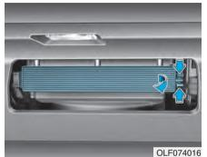
3. Remove the climate control air filter case by pulling out the right
