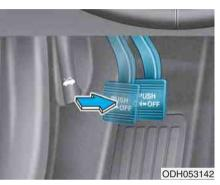
Always set the parking brake before leaving the vehicle, to apply:
