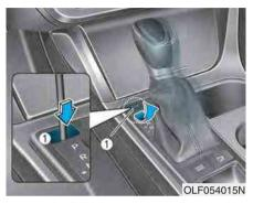
If the shift lever cannot be moved from the P (Park) position into R (Reverse) position with the brake pedal depressed, continue depressing the brake, and then do the following:
