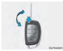
Press the release button then the key will unfold automatically.
