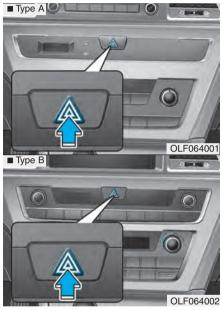
The hazard warning flasher serves as a warning to other drivers to exercise extreme caution when approaching, overtaking, or passing your vehicle. It should be used whenever emergency repairs are being made or when the vehicle is stopped near the edge of a roadway.
