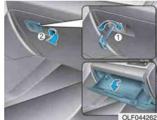
The glove box can be locked and unlocked with the mechanical key (1).
