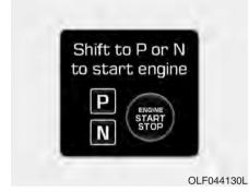
This warning message illuminates if you try to start the engine with the shift lever not in the P (Park) or N (Neutral) position.
