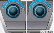
The temperature will increase to the maximum (HI) by turning the knob to the right.
