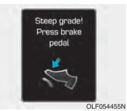
• To hold the vehicle on a hill use the foot brake or the parking brake. If the vehicle is held by applying the accelerator pedal on a hill the clutch and transmission will be overheated
