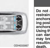
LATCH anchors have been provided in the left and right outboard rear seating positions. Their locations are shown in the illustration. There are no LATCH anchors provided for the center rear seating position.
