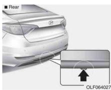
If towing is necessary, we recommend you to have it done by an authorized HYUNDAI dealer or a commercial tow truck service. If towing service is not available in an emergency, your vehicle may be temporarily towed using a cable or chain secured to the emergency towing hook at the rear of the vehicle.
