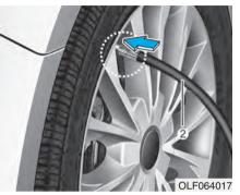
4. Unscrew the valve cap from the valve of the flat tire and screw the filling hose (2) of the sealant bottle onto the valve.
