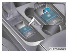
To apply the EPB (Electric Parking Brake):
