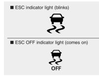
When the ignition switch is placed to the ON position, the ESC indicator light illuminates, then goes off if the ESC system is operating normally.
