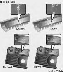
A vehicle's electrical system is protected from electrical overload damage by fuses.
