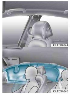
Curtain air bags are located along both sides of the roof rails above the front and rear doors. They are designed to help protect the heads of the front seat occupants and the rear outboard seat occupants in certain side impact collisions.
