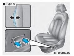
Lumbar support (for driver's seat, if equipped) To adjust the lumbar support:
