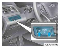
When the vehicle's parking lights or headlights are on, press the illumination control button to adjust the brightness of the instrument panel illumination. When pressing the illumination control button, the interior switch illumination intensity is also adjusted. The selected brightness of illumination can be saved in the Driver Position Memory System (if equipped).
