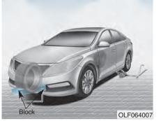
Block both the front and rear of the tire diagonally opposite of the tire you are changing.
