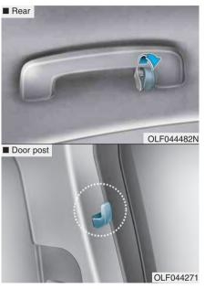
To hang items, pull the hanger down. These hangers are not designed to hold large or heavy items.
