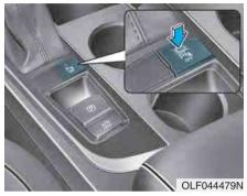
Push the button to turn off the Rear Parking Assist System. The indicator light on the button will turn on.
