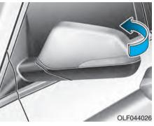
To fold the outside rearview mirror, grasp the housing of the mirror and then fold it toward the rear of the vehicle.
