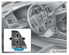
The outlet vents can be opened (R) or closed ( $\bigcirc$ ) separately using the thumbwheel.
