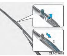
2. Lift the wiper blade clip. Then push down the blade body.
