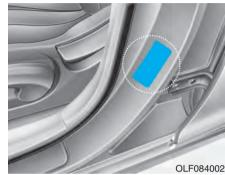
The vehicle certification label attached on the driver's side center pillar gives the Vehicle Identification Number (VIN).
