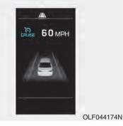
This mode displays the state of the Smart Cruise Control (SCC) and Lane Departure Warning System (LDWS).
