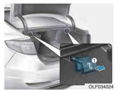
3. Pull on the seatback folding lever (1) located in the trunk.
