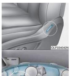
Your vehicle is equipped with a side air bag in each front seat. The purpose of the air bag is to provide the vehicle's driver and the front passenger with additional protection than that offered by the seat belt alone.
