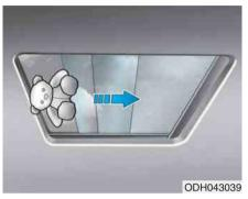
If the sunroof senses any obstacle while it is closing automatically, it will reverse direction then stop to allow the object to be cleared.
