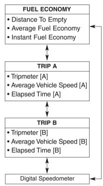
To change the trip mode, rotate the MOVE switch " $\blacktriangle$  ,  $\blacktriangledown$ " on the steering wheel.
