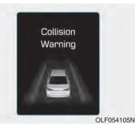
A warning message and chime will be provided when rapidly approaching a slower moving, braking or stopped vehicle ahead.
