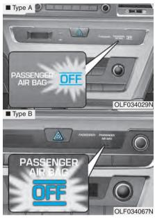
Your vehicle is equipped with an Occupant Classification System (OCS) in the front passenger's seat.
