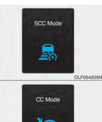
The sensitivity of vehicle speed when following the front vehicle to maintain the set distance can be adjusted. Go to the User Settings Mode (Driving Assist) and select SCC (Smart Cruise Control). You may select one of the three stages you prefer.
