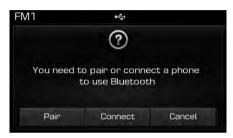
If *Bluetooth*<sup>®</sup> Wireless Technology devices are paired but none are currently connected, pressing the **PHONE** key or the key on the steering wheel displays the following screen. Press the [Pair] button to pair a new device or press the [Connect] to connect a previously paired device.
