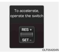
In traffic, your vehicle will stop if the vehicle ahead of you stops. Also, if the vehicle ahead of you starts moving, your vehicle will start as well. However, if the vehicle stops for more than 3 seconds, you must depress the accelerator pedal or push up the lever (RES+) to start driving.
