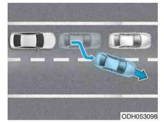
When vehicles are at a standstill and the vehicle in front of you changes to the next lane, be careful when your vehicle starts to move because it may not recognize the stopped vehicle in front of you.
