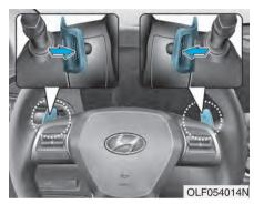
The paddle shifter is available when the shift lever is in the D (Drive) position or Sports Mode. With the shift lever in the D position
