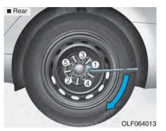
14. Use the wheel lug nut wrench to tighten the lug nuts in the order shown. Double-check each lug nut until they are tight. After changing tires, have an authorized HYUNDAI dealer tighten the lug nuts to their proper torque as soon as possible. **The wheel lug nut should be tightened to 65~79 lb.ft (9~11 kg.m).**
