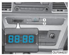
Whenever the battery terminals or related fuses are disconnected, you must reset the time.
