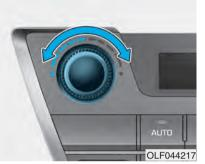
2. Turn the temperature control knob to the desired temperature. If the temperature is set to the lowest setting (Lo), the air conditioning system will operate continuously. To turn the automatic operation off, select any button of the following:
