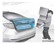
On a vehicle equipped with a smart key, the trunk can be opened using the Smart Trunk system.
