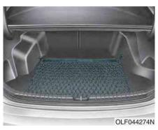
To keep items from shifting in the trunk, you can use the 4 holders located in the trunk to attach the luggage net.
