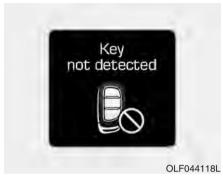
This warning message illuminates if the smart key is not detected when you press the Engine Start/Stop button.
