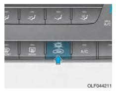
This button is used to select the outside (fresh) air position or recirculated air position.
