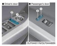
When pressing the  $(\bigcirc)$  switch (1), all vehicle doors will lock.
