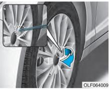
6. Insert the flat tip on the jack handle (or screwdriver) into the groove of the wheel cap and pry gently to remove the wheel cap (If equipped).
