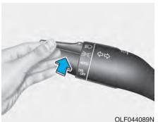
To turn on the high beam headlamp, push the lever away from you. The lever will return to its original position. The high beam indicator will light when the headlamp high beams are switched on.
