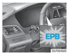
If the EPB Malfunction Indicator remains on, comes on while driving, or does not come on when the Engine Start/Stop button is in the ON position, this indicates the EPB may have malfunctioned. Have your vehicle checked by an authorized HYUNDAI dealer as soon as possible.
