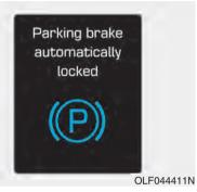
**Parking brake automatically locked** When the EPB is applied from Auto Hold, a warning will sound and a message will appear.
