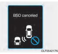
The message will appear to notify the driver if there are foreign substances on the rear bumper. The light on the switch and the system will turn off automatically.
