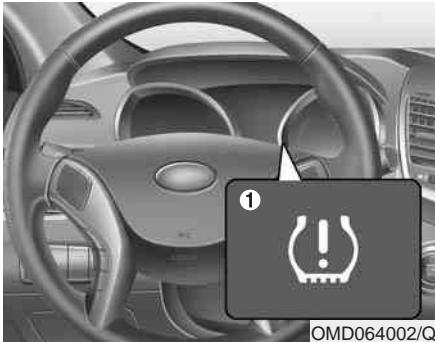
(1) Low Tire Pressure Telltale/ TPMS Malfunction Indicator
