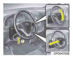
To change the steering wheel angle, pull down the lock-release lever (1), adjust the steering wheel to the desired angle (2) and the desired position (if equipped) (3), then pull up the lock-release lever to lock the steering wheel in place. Be sure to adjust the steering wheel to the desired position before driving.
