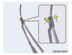
2. Press the button and slide the blade assembly upward.
