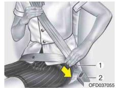
3. Pull the webbing and insert the tongue plate (1) into the open end of the buckle (2) until an audible "click" is heard, indicating the latch is locked. Make sure the belt is not twisted
