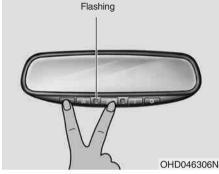
1. When programming the buttons for the first time, press and hold the left and center buttons (♠,♠) simultaneously until the indicator light begins to flash after approximately 20 seconds. (This procedure erases the factory-set default codes. Do not perform this step to program additional hand-held transmitters.)
