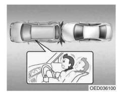
Frontal air bags are not designed to inflate in rear collisions, because occupants are moved backward by the force of the impact. In this case, inflated air bags would provide additional occupant protection.
