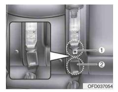
2. Insert the metal tab (1) into the open end of the anchor connector (2) until an audible "click" is heard, indicating the latch is locked. Make sure the belt is not twisted.
