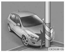
Air bags may not inflate if the vehicle collides with objects such as a utility pole or a tree, where the point of impact is concentrated and the collision energy is absorbed by the vehicle structure. C041100AFD
