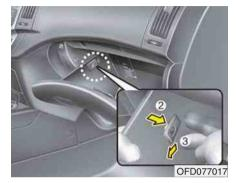
With the glove box open, remove the stoppers on both sides to allow the glove box hang freely on the hinges.
