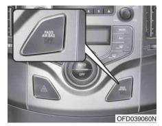
If the front passenger seat is occupied by a person that the system determines to be of adult size, and he/she sits properly (sitting upright with the seatback in an upright position, centered on the seat cushion with their seat belt on, legs comfortably extended and their feet on the floor), the "PASSENGER AIR BAG OFF" or "PASS AIR BAG OFF" indicator will be turned off and the front passenger's air bag will be able to inflate, if necessary, in frontal crashes.
