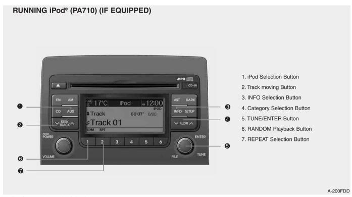
In case the iPod exclusive cable is connected to the multimedia jack inside the consol on the right hand side of the driver's seat. When the iPod is connected, the 'iPod' icon will be displayed on the top right corner of the display screen.
