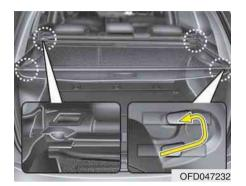
To use the cargo security screen, pull the handle backward and insert the edges into the slots.
